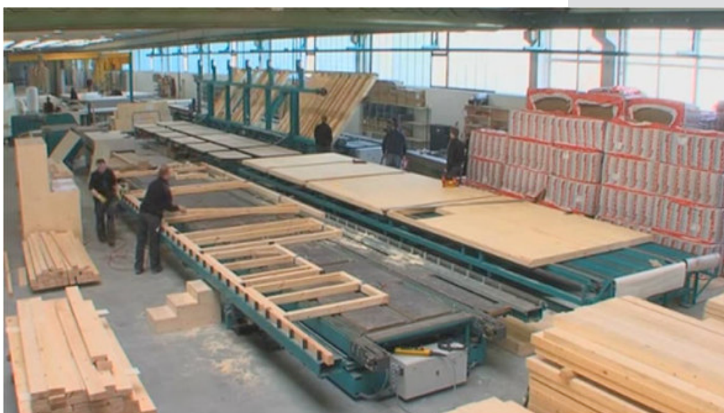
Figure 3. Example of process to production the platform frame panel.
