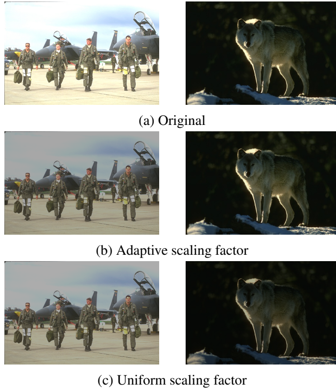
Fig. 5.5 Comparison between the proposed LABS algorithm for adaptive brightness scaling in OLED displays and a standard uniform scaling.
