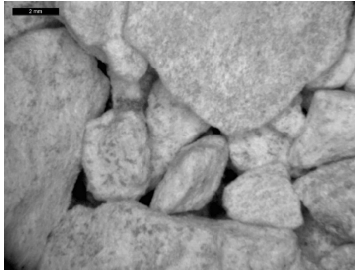
Figure 73. Microscopic imaging of quartz sand, obtained by using a video-microscope LEICA VZ85R (magnification: 40x).
