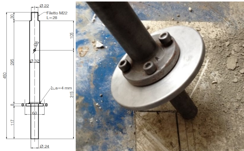
Figure 50. Schematic of the Drive Shaft (left) and photograph of the disc on the drive shaft (right).
