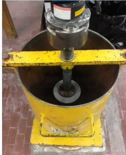
Figure 49. Detail of the disc assembled on the drive shaft inside the tank.
