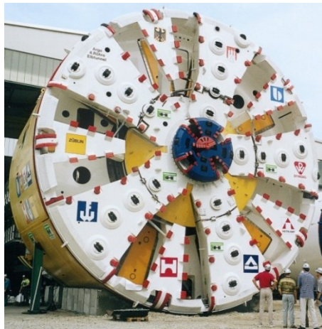
Figure 3. Cutterhead of EPB machine.
