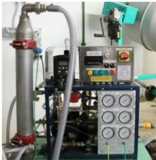
Figure 17. Lab scale foam generator at the Politecnico di Torino Laboratory.
