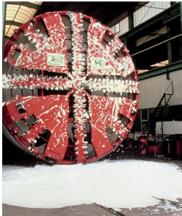
Figure 2. Foam production during works assembly, EPB shield Metro Valencia, 1995 (Herrenknecht, et al., 2011).
