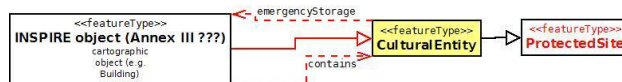
Figure 10. UML model of the new relationships between ProtectedSite and other cartographic objects
