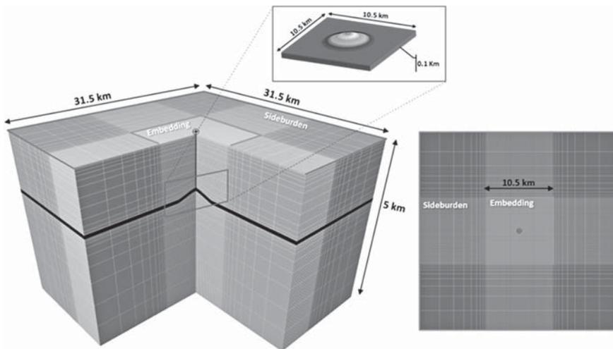
Fig. 3. Example of 3D numerical model for geomechanical simulations.
