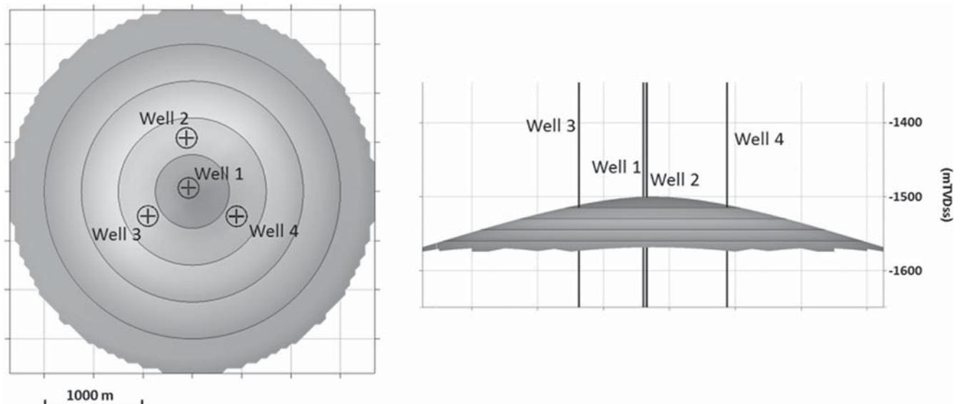
Fig. 4. Top geometry of the reservoir.
