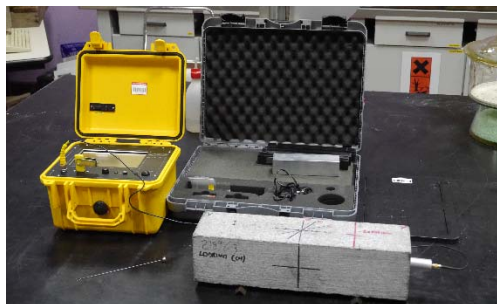
Fig. 1 Resonance Frequency meter 58-E0035/C.
