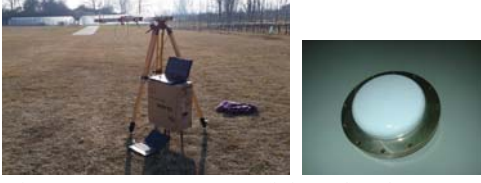
Figure 2. Measurement setup (left panel) and Antcom antenna (right panel).
