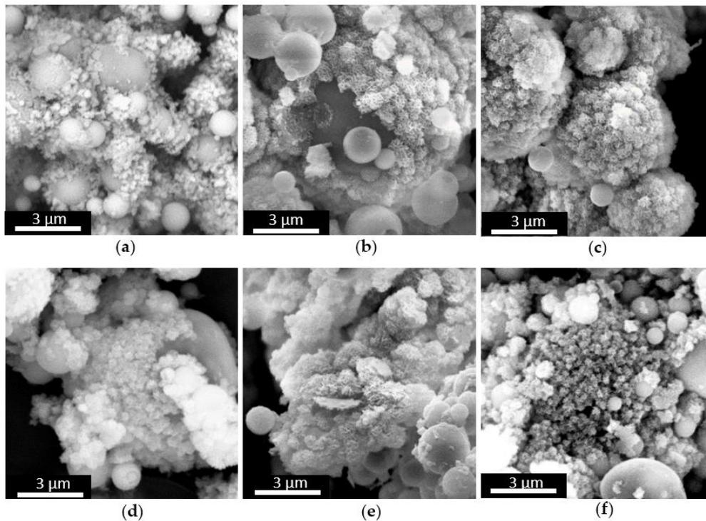
**Figure 5.** FESEM images and XRD spectra of MBG\_Sr\_SD after different time of soaking in SBF: (a) MBG\_Sr2%\_SD after 1 day; (b) MBG\_Sr2%\_SD after 3 days; (c) MBG\_Sr2%\_SD after 7 days; (d) MBG\_Sr4%\_SD after 1 day; (e) MBG\_Sr4%\_SD after 3 days; (f) MBG\_Sr4%\_SD after 7 days.
