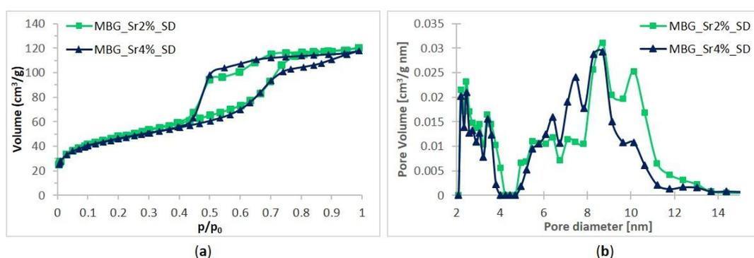
**Figure 3.** N<sub>2</sub> adsorption-desorption curves of MBG\_Sr2%\_SD and MBG\_Sr4%\_SD: (a) isotherms; (b) DFT pore size distributions.
