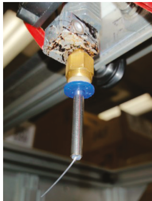
Figure 11. Wire feed guide tube. As shown, a standard M6 4.0 mm press fitting accommodates the standard threading in the hot-zone of a standard hexagon 12 V hot end. 304 stainless tubing press fits similar to a 4.0 mm PTFE tubing. Scrap PTFE tubing is fixtured to the exit zone of the 304 stainless tubing to reduce the friction associated with wire wrapping processes.
