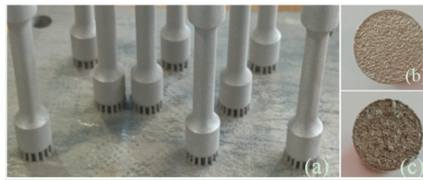
Figure 3. Support structures (a); and top (b); bottom (c) surface texture.
