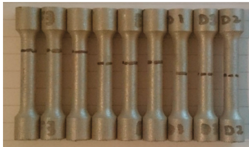
Figure 10. Customised specimen set failure points.
