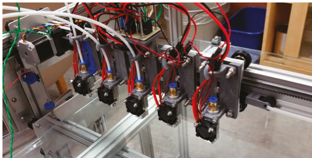
Figure 2. X-axis gantry assembly. 5 × Hexagon Full-Metal 12 V hot ends are shown fixtured to their respective ‘Z-Height Bed Leveling Adjustment’ part files. As shown, dovetail leveling mechanisms are attached to the machined aluminum plate (3.175 mm × 25.4 mm × 295.75 mm) with Hexagon nozzle diameter cylindrical axis spaced 55 mm.
