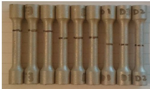
Figure 10. Customised specimen set failure points.
