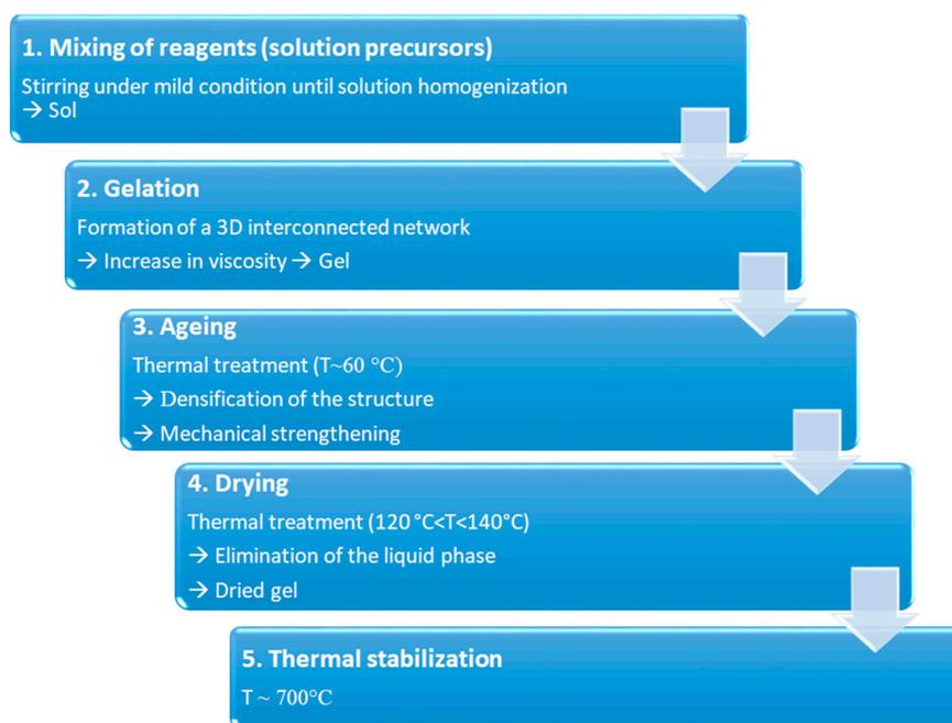
**Figure 4.** Schematization of the sol–gel process for the production of BGs.
