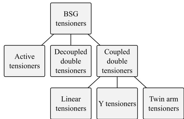
**Figure 3.** Classification of tensioning solutions for BSG-based systems.
