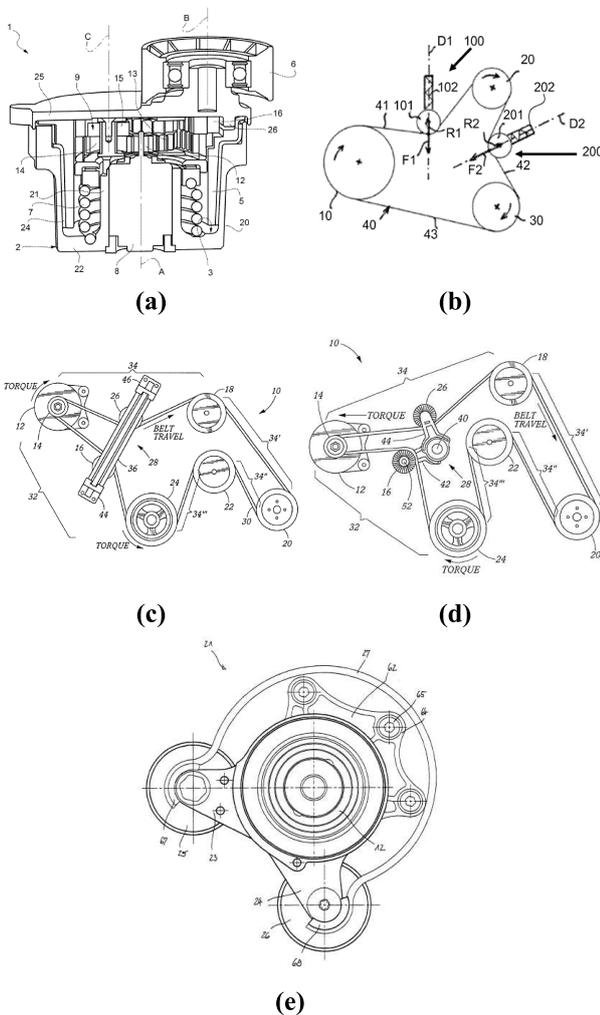
**Figure 2.** Different tensioning solutions for BSG Systems: (a) active tensioner by Dayco Europe S.r.l.;<sup>14</sup> (b) double tensioner by PSA Peugeot Citroen;<sup>15</sup> (c) linear tensioner by The Gates Corporation;<sup>16</sup> (d) Y tensioner by The Gates Corporation;<sup>17</sup> (e) rotary twin arm tensioner by Mubea Muhr und Bender KG.<sup>18</sup> The images were taken from the cited patents.
