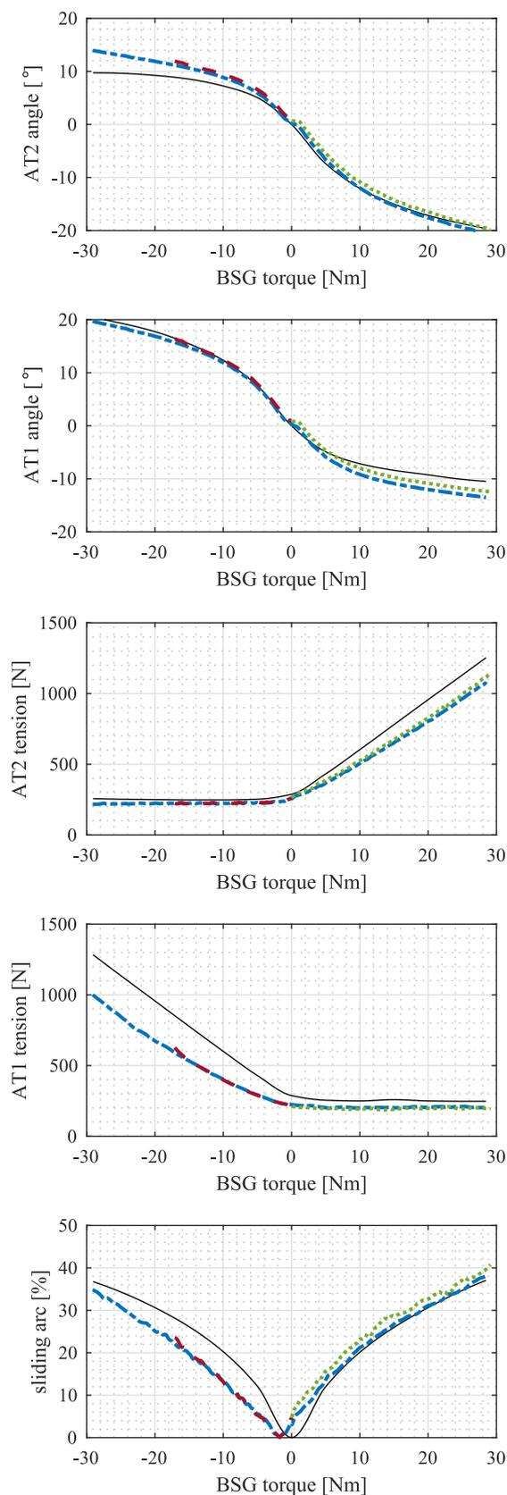
**Figure 9.** Results of a twin arm tensioning device working on a BSG-based BDS in motor and generator modes. The considered variables are the angular displacement of the tensioner pulleys, the belt span tensions and the sliding arc on the BSG pulley. Numerical results (solid) are compared to experimental data obtained at 860 rpm (dot), 2500 rpm (dash-dot) and 3800 rpm (dash).
