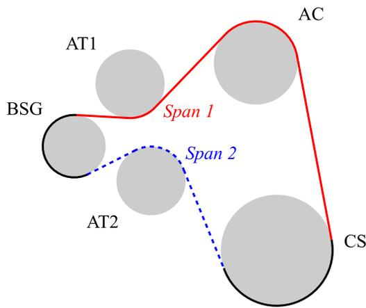
**Figure 1.** BDS layout mounting a BSG. The two belt spans are alternately tight and slack according to the operating mode of the BSG and require a dedicated tensioner (pulleys AT1 and AT2) to keep a suitable belt tension. The layout also presents crankshaft (CS) and air conditioning compressor (AC) pulleys.
