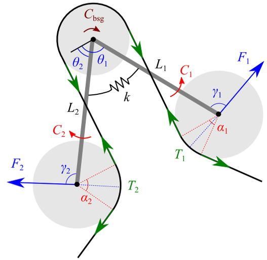
**Figure 4.** Scheme of the tensioner with variables and parameters of interest: belt tension  $T_i$ , arm force  $F_i$ , pulley wrap angle  $\alpha_i$ , force angle  $\gamma_i$ , arm torque  $C_i$ , arm angle  $\theta_i$ , arm length  $L_i$ , tensioner spring stiffness  $k$ , BSG torque  $C_{\text{bsg}}$ .
