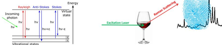
The frequencies of Raman scattered photons bring specific chemical information about the sample. Raman spectroscopy belongs to untargeted fingerprint technologies. This technique can be used for compositional sensing based on the specificity of the pattern of signals present in the Raman spectrum. Quantitative information can be obtained, after calibration, based on the Beer-like correlation between intensity and amount of substance.
