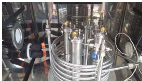
Fig. 8. Measurement chamber of the CETIAT humidity generator.
