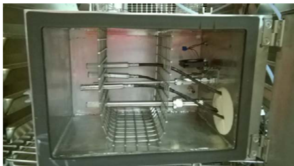
Fig. 5. Photograph showing humidity probes in the measurement chamber of the VTT MIKES calibration setup. The metal outlet tube is in the middle.
