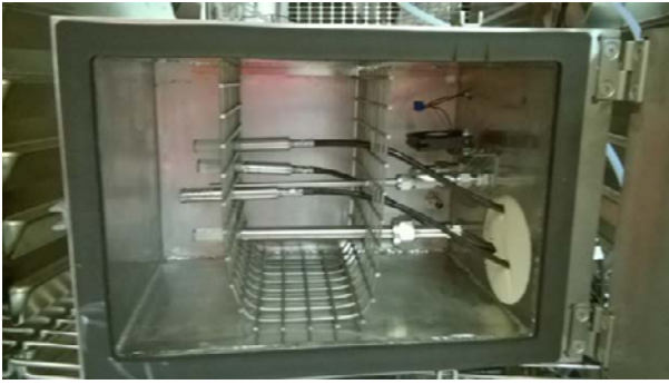
Fig. 5. Photograph showing humidity probes in the measurement chamber of the VTT MIKES calibration setup. The metal outlet tube is in the middle.
