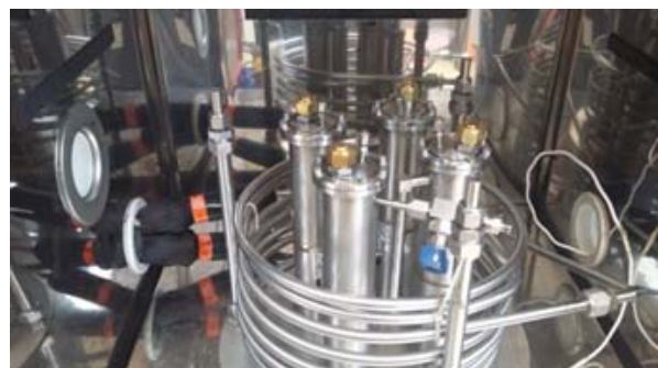
Fig. 8. Measurement chamber of the CETIAT humidity generator.
