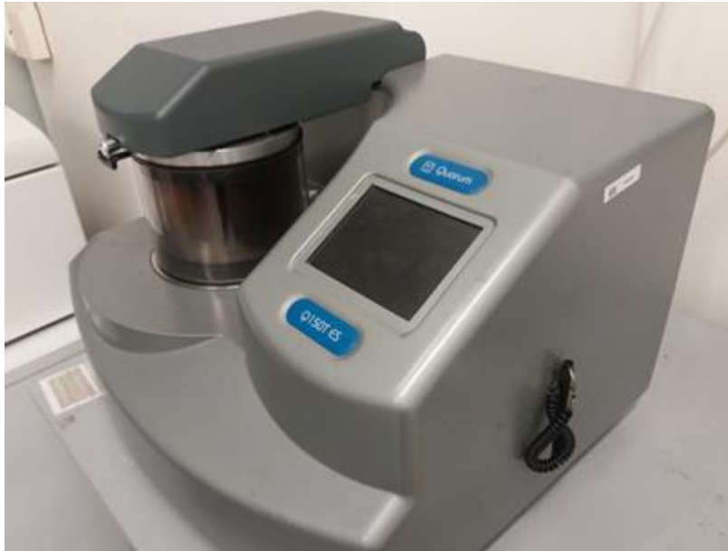
Figure 29. Sputter coater used for the silver deposition
