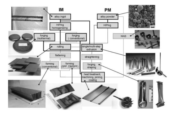
Figure 8: Processing of TiAl based alloys on an industrial scale [17].
