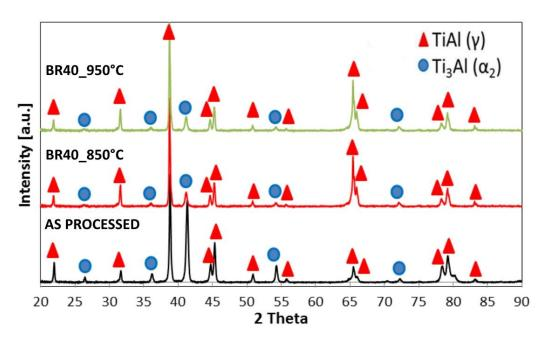
Figure 86: XRD patterns of substrate: as-processed Ti-48Al-2Cr-2Nb, and after oxidation in Burner Rig for 40 cycles at 850 or 950°C [107].
