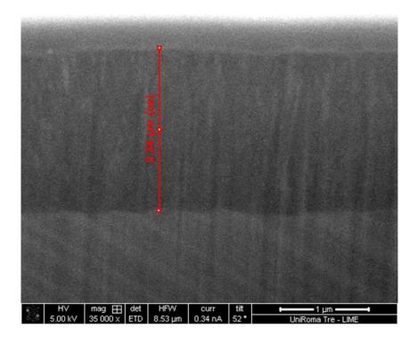
Figure 51: Cross-section of TiAlN2 sample.
