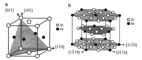
Figure 6: Cristal structures: a)  $\gamma$ -TiAl has L1<sub>0</sub> structure (ordered face centered tetragonal), and b)  $\alpha_2$ -Ti<sub>3</sub>Al has DO<sub>19</sub> structure (hexagonal closed packed) [4].
