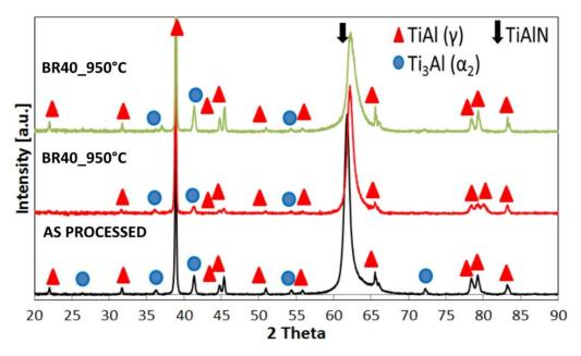
Figure 87: XRD patterns of TiAlN coated specimens (TiAlN1 coating): as-processed and after oxidation in Burner Rig for 40 cycles at 850 or 950°C [107].
