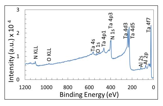
Figure 116: Survey spectrum of as-processed sample with TaAlN coating.
