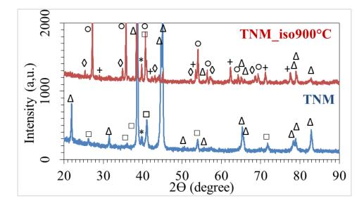
Figure 77: XRD patterns of Ti-43.5Al-4Nb-1Mo alloy: blue spectrum= as-processed, red spectrum= oxidized at 900 °C. Crystalline phases:  $\Delta$  TiAl ( $\gamma$ ), \* TiAl ( $\beta$ ),  $\Box$  Ti3Al ( $\alpha_2$ ),  $\Diamond$  Al<sub>2</sub>O<sub>3</sub> ( $\alpha$ ),  $\circ$  TiO<sub>2</sub>, + NbO [102].
