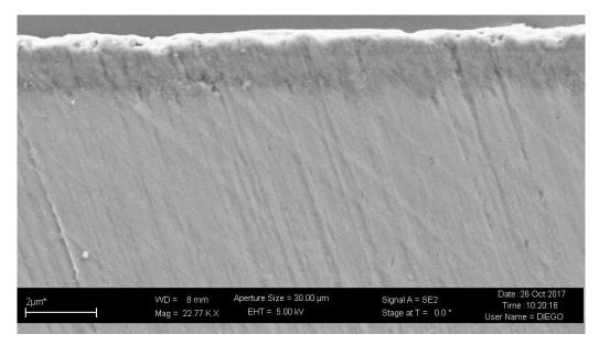
Figure 108: SEM imagine of cross-section of uncoated 48-2-2 intermetallic alloy after oxidation at 900  $^{\circ}$ C for 30 minutes (oxide layer a bit less than 2 µm thick).
