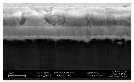
Figure 112: SEM cross-section imagine of TaAlN coated sample after oxidation at 900°C for 30 min (the up layer is an oxide scale about 2  $\mu$ m thick grown on remaining TaAlN coating 1.2  $\mu$ m thick, and the lower layer is the TiAl interlayer about 0.4  $\mu$ m thick).
