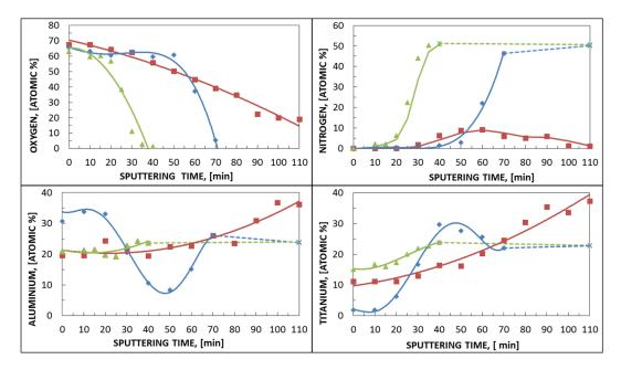
Figure 103: XPS depth profiles, after 200 thermal cycles at 950 °C: red line = TiAl (uncoated alloy), blue line = TiAlN1 coated sample, green line = TiAlN3 coated sample. The dashed lines show the extrapolation of the curves toward the concentration of titanium, aluminium and nitrogen found in the TiAlN coatings [125].
