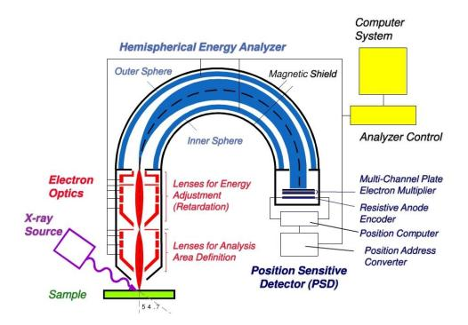
The schematic operating principle of XPS technique is shown in Figure 64.
