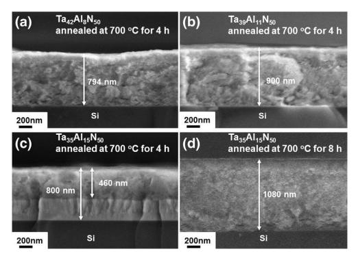
Figure 41: Cross-sectional SEM images of Ta-Al-N coatings after isothermal oxidation at 700°C: (a)  $Ta_{42}Al_8N_{50}$ , (b)  $Ta_{39}Al_{11}N_{50}$ , (c)  $Ta_{35}Al_{15}N_{50}$ , and (d)  $Ta_{35}Al_{15}N_{50}$  [96].
