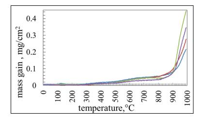
Figure 70: TGA curves of TiAl alloys recorded under 50 ml/min air flow during heating from 25 to 1000 °C at 5°/min: Ti-48Al-2Cr-2Nb (green line), Ti-48Al-2Nb-0.7Cr-0.3Si (violet line), Ti-43.5Al-4Nb-1Mo (red line), and Ti-47Al-2Cr-8Nb (blue line) [102].
