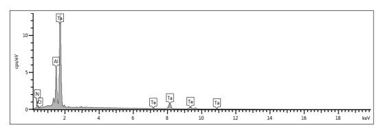
Figure 109: EDS spectrum of surface of as-processed TaAlN coated sample.
