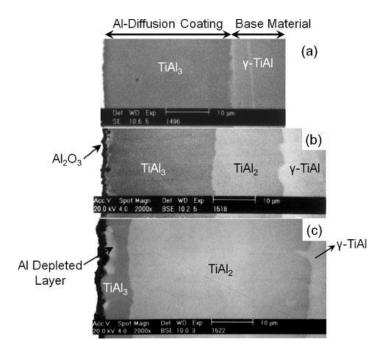
Figure 24: SEM cross section of  $\gamma$ -TiAl alloy aluminised at 800 °C for 5 h in a low Al activity pack: a) as processed, b) after 10h isothermal oxidation at 900 °C and c) after long term oxidation of 100h at 900 °C [59].
