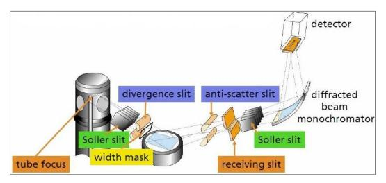
A schematic description of XRD equipment is shown in Figure 58.
