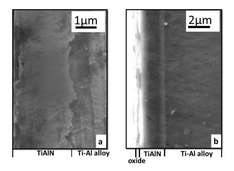
Figure 96: SEM imagines of TiAlN1 cross-section: (a) before and (b) after 200 cycles at 950 °C in Burner Rig apparatus.
