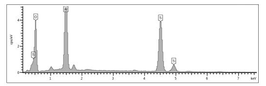
Figure 105: EDS of Ti-48A1-2Cr-2Nb oxidized at 900°C for 30 min.
