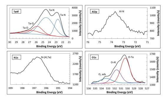
Figure 118: XPS HR spectra of as-processed samples with TaAlN coating.
