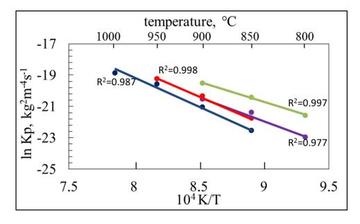
Figure 83: Arrhenius plot for oxidation of Ti-48Al-2Cr-2Nb (green line), Ti-48Al-2Nb-0.7Cr-0.3Si (violet line), Ti-43.5Al-4Nb-1Mo (red line), and Ti-47Al-2Cr-8Nb (blue line) [102].
