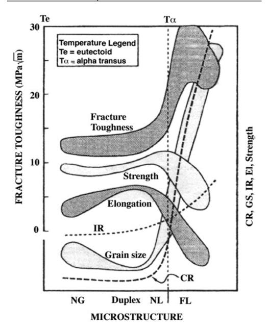
Figure 19: Dependence of mechanical properties (fracture toughness, strength, ductility, impact resistance, creep resistance) and grain size on the microstructure (Near Gamma, Duplex, Nearly lamellar, Fully Lamellar) [4].
