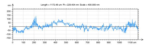
Figure 48: Roughness profile of TiAlN2 sample surface before coating deposition.
