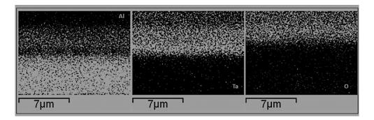
Figure 113: EDS cross-section of sample with TaAlN coating oxidized at 900°C for 30 minutes.
