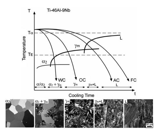
Figure 11 : CCT diagram of a Ti-46Al-9Nb alloy and different microstructures formed at specific cooling rates (FC-furnace cooling, AC-air cooling, OC-oil cooling, WC-water cooling) [17].
