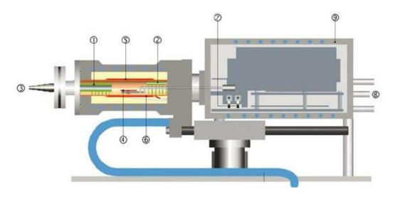
Figure 66: Schematic Thermogravimetric apparatus Metter Toledo, comprising: 1baffles, 2-reactive gas capillary, 3-gas outlet, 4-temperature sensors, 5-furnace heater, 6furnace temperature sensor, 7-adjustment ring weights, 8-protective and purge gas connector, 9-thermostated balance [134].
