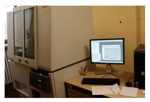
Figure 57: X'PERT PRO PW3040/60 located at politecnico di Torino (DISAT).
