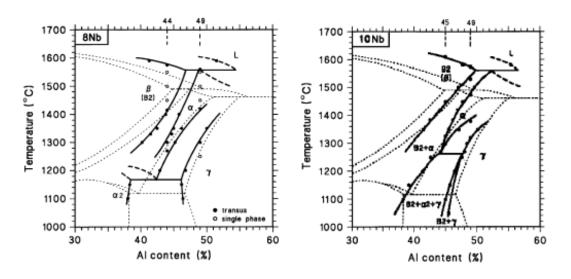
Figure 13: Ti-Al quasi phase diagrams with Nb (8% at.) and Nb (10% at.) [23].
