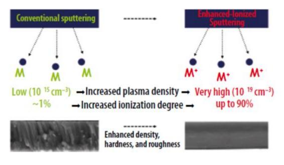
Figure 45: Magnetron Sputtering and High Power Impulse Magnetron Sputtering schematic processes [117].
