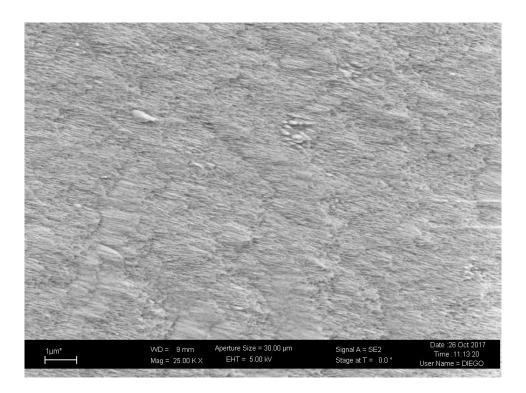
Figure 111: SEM surface imagine of TaAlN coated sample after oxidation at 900°C for 30 minutes.
