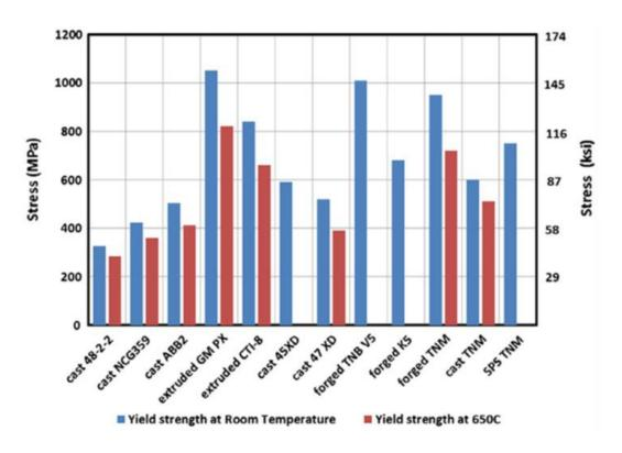
Figure 20: Yield strengths of TiAl-based alloys at room temperature and at 650°C [3].
