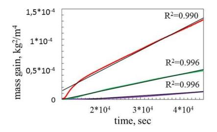
Figure 79: TGA data (50 ml/min in air for 10 h) of Ti-48Al-2Cr-2Nb alloy fitted at different temperatures with straight lines according to a parabolic law: violet line= 800 °C, green line= 850 °C and red line= 900 °C [102].
