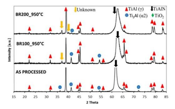
Figure 99: XRD patterns of TiAlN1 samples before and after 100 and 200 oxidation cycles in burner rig [125].
