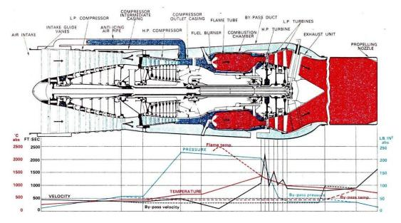
Figure 1: Design process of gas turbine engine: estimated temperature, velocity and pressure [1].
