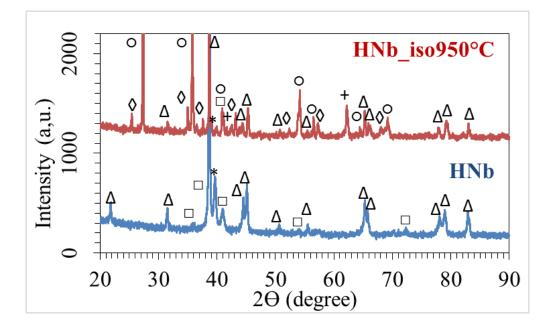
Figure 78: XRD patterns of Ti-47Al-2Cr-8Nb alloy: blue spectrum= as-processed, red spectrum= oxidized at 950 °C. Crystalline phases:  $\Delta$  TiAl ( $\gamma$ ), \* TiAl ( $\beta$ ),  $\Box$  Ti3Al ( $\alpha_2$ ),  $\Diamond$  Al<sub>2</sub>O<sub>3</sub> ( $\alpha$ ),  $\circ$  TiO<sub>2</sub>, + NbO [102].
