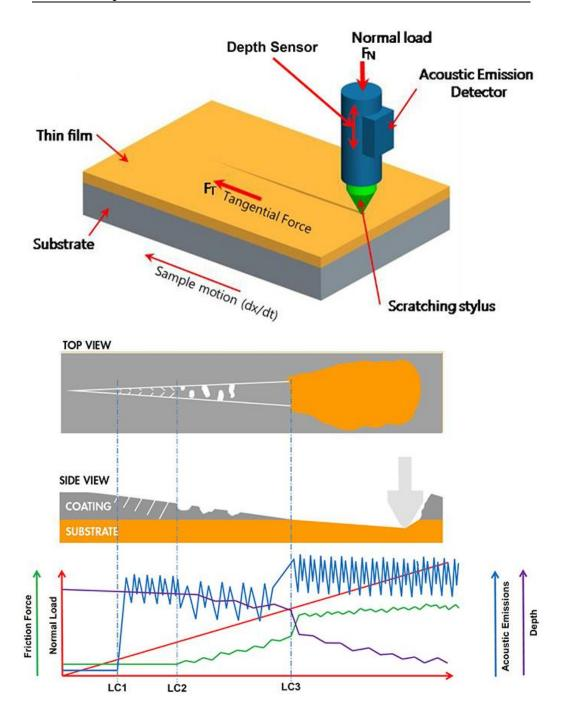
Figure 69: Progressive Load Scratch Test [136], [137].
