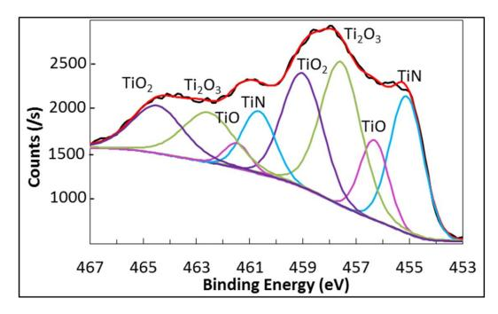
Figure 95: Fitting of Ti2p complex HR spectrum, detected for TiAlN1 sample after 40 burner rig cycles at 850°C [107].
