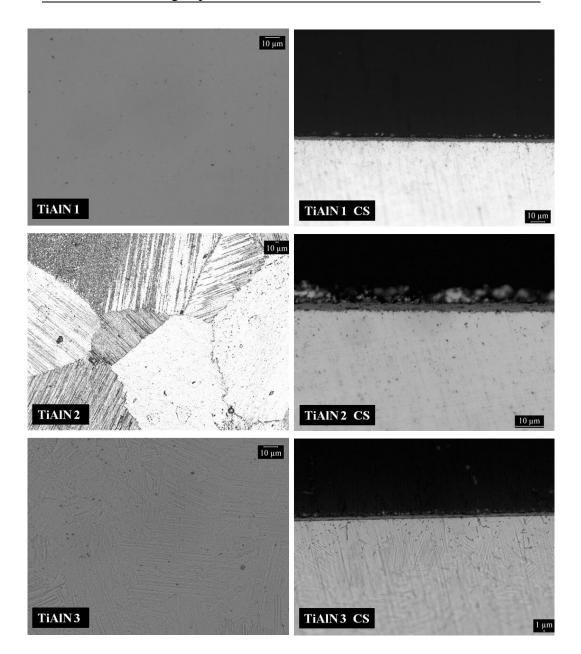
Figure 53: SEM imagines. Microstructures of TiAlN coatings (top and cross-section).
