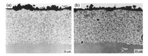
Figure 32: Cross section of Ti-50Al-10Cr (at.%) coating deposited on Ti-50Al (at.%): a) after exothermal oxidation-1000 h of at 900° C, b) after 100 cycles at 1000°C [65].
