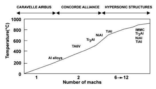
Figure 2: Expected performance of structural alloys developed for aircraft: temperature and speed [4].
