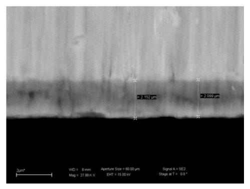
Figure 55: SEM cross-section of TaAlN coating.
