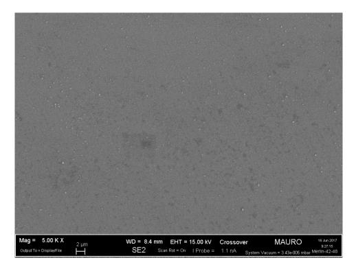
Figure 54: SEM image of TaAlN coating microstructure.
