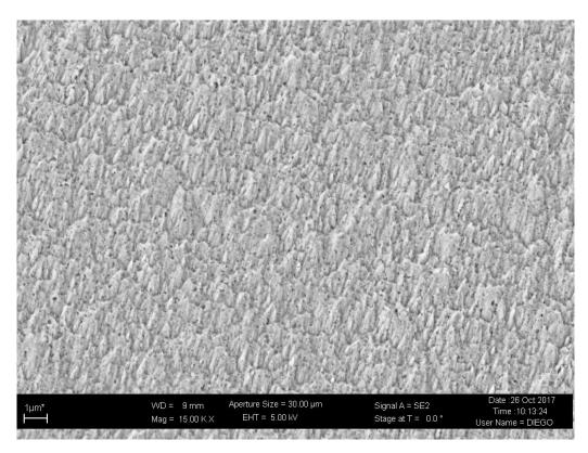
Figure 107: SEM imagine of surface of intermetallic alloy after oxidation at 900°C for 30 minutes.
