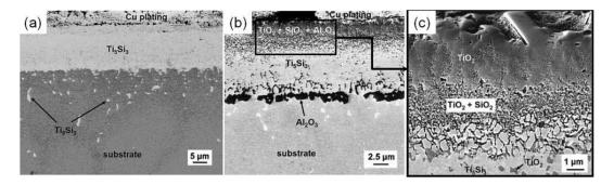
Figure 23: SEM micrograph of Si-based coating deposited on TiAl alloy: (a) after 100h at  $1000^{\circ}$ C ( $10^{-6}$  mbar), (b) and (c) after 1000 cycles at 950 °C in air [38].
