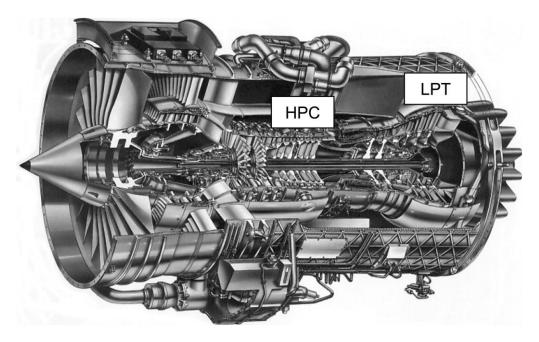
Figure 3: BR 715 aero engine. High Pressure Compressor (HPC) and Low Pressure Turbine (LPT) [6].
