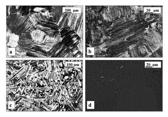
Figure 44: Optical microscopy images: (a) a fully lamellar microstructure of Ti-48Al-2Cr-2Nb, a near lamellar microstructure of (b) Ti-47Al-2Cr-8Nb and (c) Ti-48Al-2Nb-0.7Cr-0.3Si. SEM image (d): a near lamellar microstructure of Ti-43.5Al-4Nb-1Mo [102].
