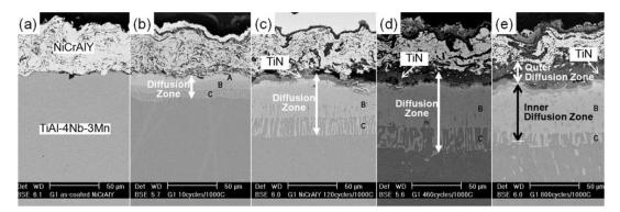
Figure 27: SEM (a) as-processed NiCrAlY coated TiAl-4Nb-3Mn (% at.) alloy, (b) oxidized after 10 cycles and (c) 120 cycles, (d) 460 cycles (e) 800 cycles at 1000°C [69].
