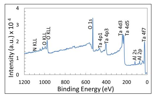
Figure 117: Survey spectrum of sample with TaAlN coating oxidised at 900°C for 30 min.
