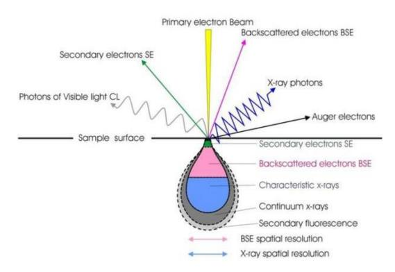
Figure 61: Schematic principle of SEM. X-ray interaction with the atoms of sample [130].
