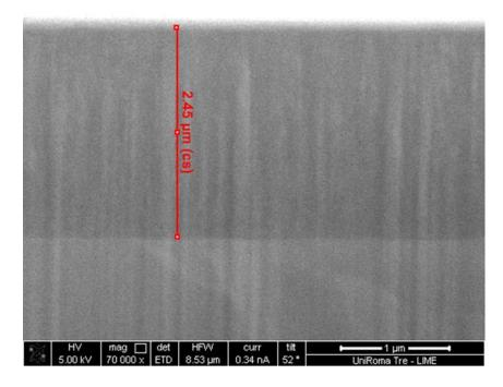
Figure 50: Cross-section of TiAlN1 sample.
