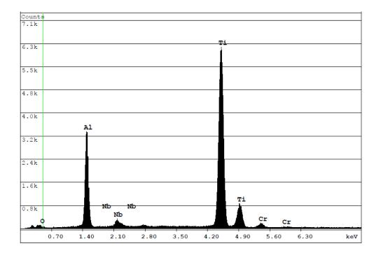
Figure 104: EDS of as-processed Ti-48Al-2Cr-2Nb surface.
