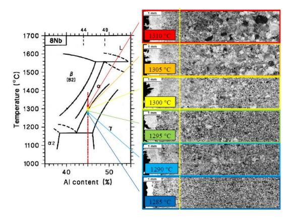
Figure 15: The microstructure of Ti-45Al-2Cr-8Nb alloy obtained by heat treatment at different temperatures in the vicinity of  $T\alpha = 1295$  °C. The yellow dotted line indicates the border (2mm) [21].
