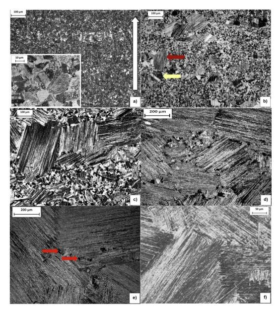
Figure 18: Optical microscopy images of Ti-48Al-2Nb-0.7Cr-0.3Si microstructure:
