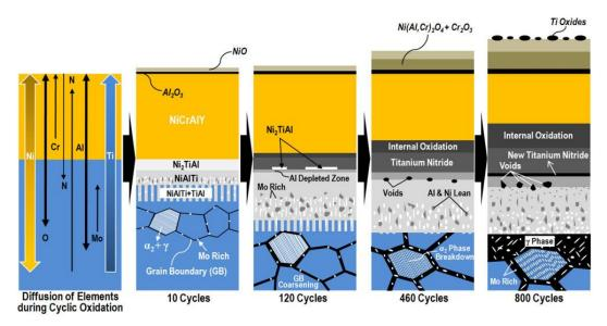
Figure 29: Diffusion processes occurring in NiCrAlY coated TiAl-4Nb-3Mn (% at.) alloy during cycling oxidation at 1000°C [70].
