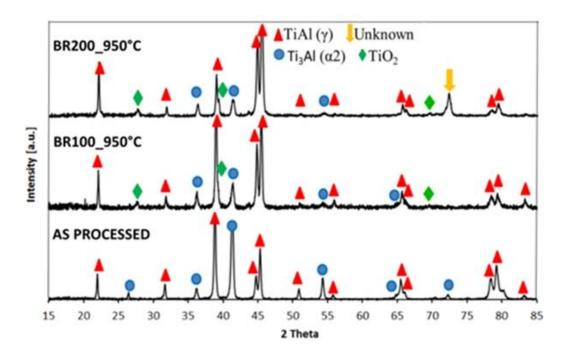
Figure 98: XRD patterns of TiAl substrate before and after 100 and 200 oxidation cycles in burner rig [125].
