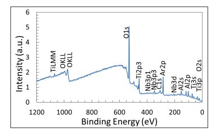
Figure 90: XPS survey spectrum of TiAl substrate oxidized in Burner Rig (40 cycles at 950 °C), after argon surface cleaning.
