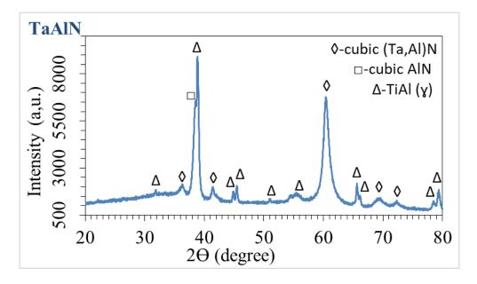
Figure 114: XRD plot of surface of as-processed samples with TaAlN coating.
