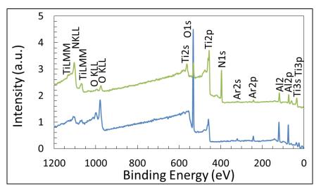
Figure 92: XPS survey spectra of oxidized coatings after 40 cycles at 950°C in burner rig: TiAlN1 (blue line) and TiAlN3 (green line), after surface cleaning [107].
