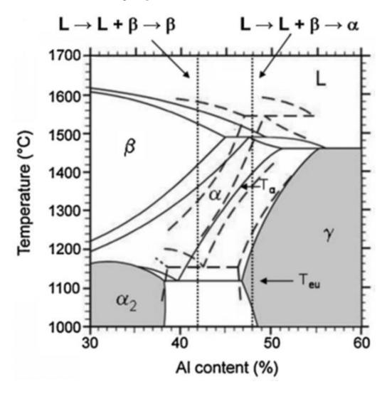
Figure 7: Section of the binary Ti–Al-phase diagram (continuous lines). Tα: αtransus temperature; Teu: eutectoid temperature. Two vertical dotted lines markered the range of the technical γ-TiAl based alloys (45-48 % at. of Al). The broken lines show the effect of Nb (8 at.%) on the position of the phase field regions [17].
