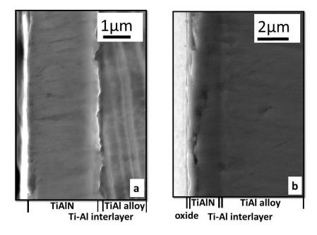
Figure 97: SEM imagines of TiAlN3 cross-section: (a) before and (b) after 200 cycles at 950 °C in Burner Rig apparatus.
