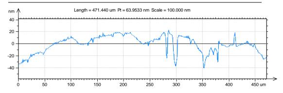
Figure 47: Roughness profile of TiAlN1 sample surface before coating deposition.
