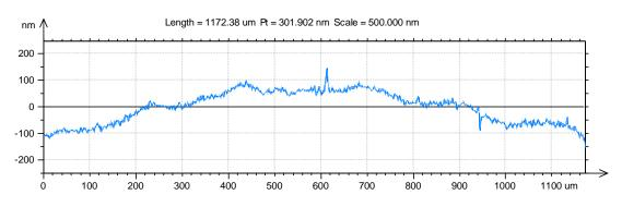
Figure 49: Roughness profile of TiAlN3 sample surface before coating deposition.
