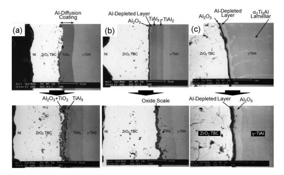
Figure 31: SEM imagines of cross-section of TBC/ γ-TiAl alloy (in up of the figure - complex system before oxidation, in down- after oxidation in air at 900 °C): a) aluminized BC, b) substrate pre-oxidation in air, c) substrate pre-oxidation in oxygen [72].
