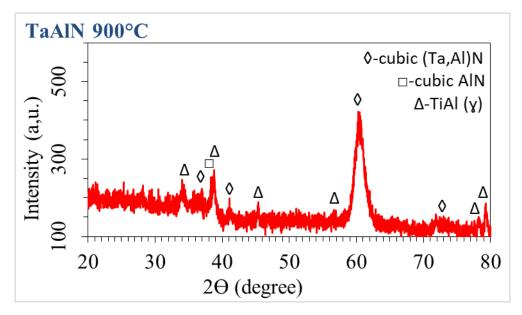
Figure 115: XRD plot of surface of with TaAlN coating after oxidation at 900°C for 30 min in air.
