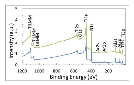
Figure 91: XPS survey spectra of as deposited coatings: TiAlN1 (blue line) and TiAlN3 (green line), after surface cleaning [107].
