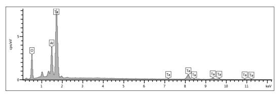
Figure 110: EDS of TaAlN coated sample after oxidation at 900°C for 30 minutes.
