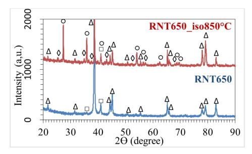
Figure 76: XRD patterns of Ti-48Al-2Nb-0.7Cr-0.3Si alloy: blue spectrum= asprocessed, red spectrum= oxidized at 850°C. Crystalline phases:  $\Delta$  TiAl ( $\gamma$ ),  $\Box$  Ti<sub>3</sub>Al ( $\alpha_2$ ),  $\Diamond$  Al<sub>2</sub>O<sub>3</sub> ( $\alpha$ ),  $\circ$  TiO<sub>2</sub> [102].
