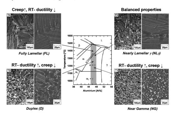
Figure 10: Microstructures of TiAl-based alloys after heat treatment [17].
