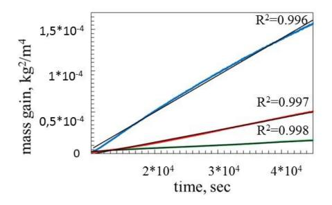
Figure 81: TGA data (50 ml/min in air for 10 h) of Ti-43.5Al-4Nb-1Mo alloy fitted at different temperatures with straight lines according to a parabolic law: green line= 850 °C, red line= 900 °C and blue line = 950 °C [102].
