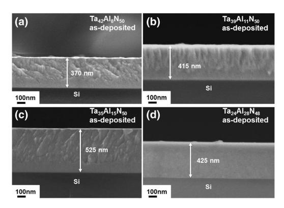
Figure 39: SEM cross-section of as-deposited coatings: (a)  $Ta_{42}Al_8N_{50}$ , (b)  $Ta_{39}Al_{11}N_{50}$ , (c)  $Ta_{35}Al_{15}N_{50}$ , and (d)  $Ta_{24}Al_{28}N_{48}$  [96].
