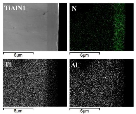
Figure 85: Cross section of TiAlN1 sample: coating morphology and nitrogen, titanium and aluminium concentration maps [107].
