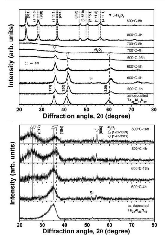
Figure 40: XRD coatings before and after isothermal oxidation at 600°C, 700°C, 800°C: (up) Ta<sub>35</sub>Al<sub>15</sub>N<sub>50</sub>, and (down) Ta<sub>24</sub>Al<sub>28</sub>N<sub>48</sub> [96].
