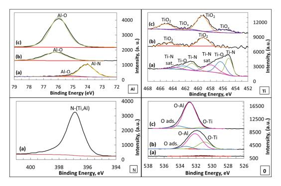
Figure 101: XPS HR spectrums of TiAlN1 sample: (a) as processed; (b) after 100 thermal cycles at 950°; (c) after 200 thermal cycles at 950°. XPS HR N1s not observed after cyclic oxidation (Curves (b) and (c) not reported) [125].
