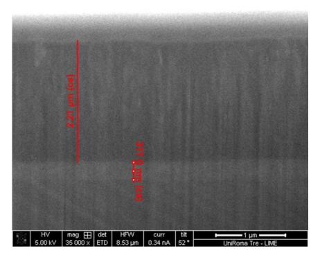
Figure 52: Cross-section of TiAlN3 sample.
