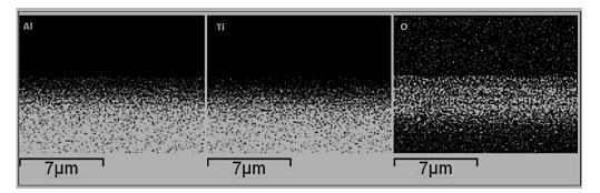
Figure 106: EDS cross-section of Ti-48A1-2Cr-2Nb oxidized at 900°C for 30 minutes.
