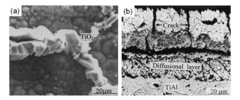
Figure 26: CoCrAlY coated γ-TiAl after 100 cycles at 1000°C: (a) surface morphology, (b) cross-section microstructure [65].
