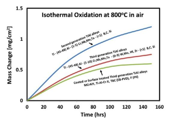
Figure 21: Oxidation behaviour of coated and uncoated TiAl alloys [3].
