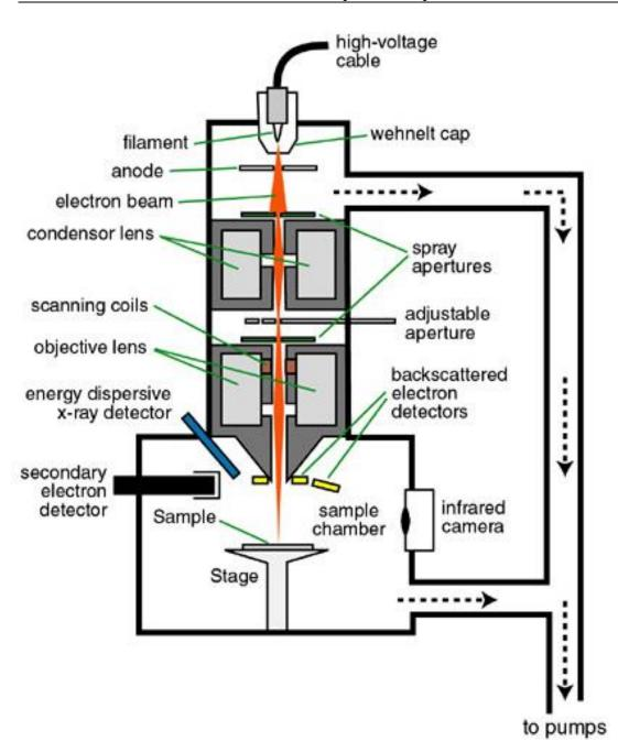
Figure 60: Schematic SEM apparatus [129].
