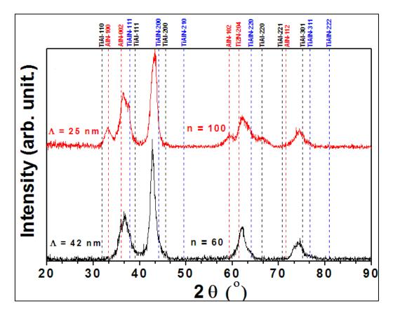
Figure 35: XRD patterns of the (Ti-Al/Ti-Al-N)<sub>n</sub> multilayer coatings deposited on silicon (100): black pattern - 60 multilayer system with a period of 42 nm, and red pattern -100 multilayer system with a period of 25 nm. The positions of TiAlN peaks (JCPDF 00-037-1140), TiAl (JCPDF 00-005-0678) and AlN (JCPDF 00-003-1144) are indicated by dash lines [87].
