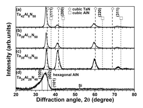
Figure 38: XRD patterns of as-deposited coatings: (a)  $Ta_{42}Al_8N_{50}$ , (b)  $Ta_{39}Al_{11}N_{50}$ , (c)  $Ta_{35}Al_{15}N_{50}$ , and (d)  $Ta_{24}Al_{28}N_{48}$  [96].
