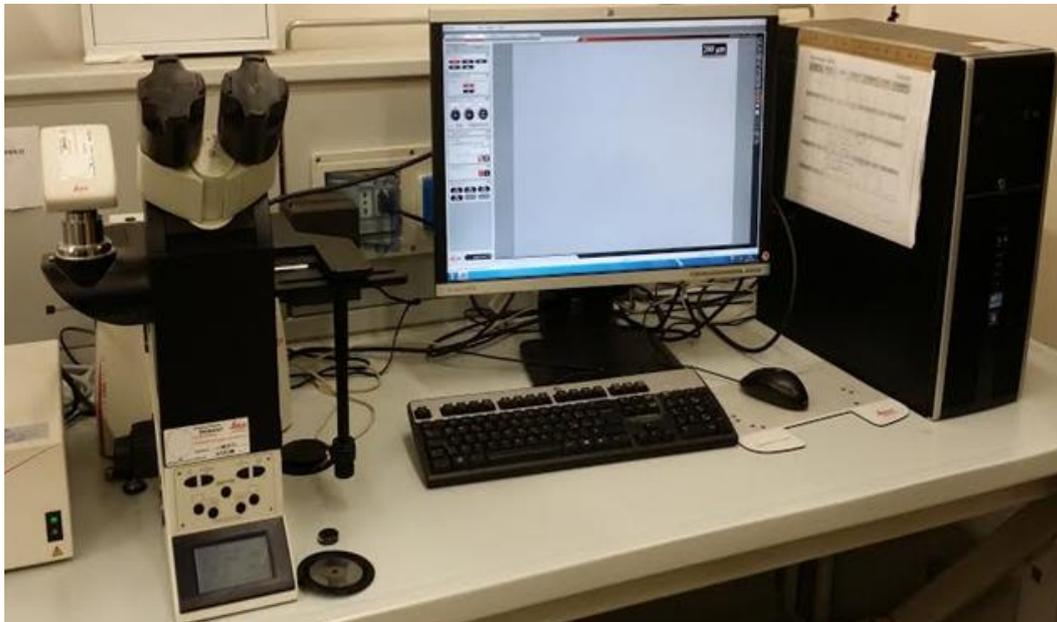
Figure 59: Leica DMI 5000 M optical microscope.
