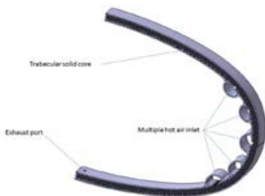
Figure 1: Schematic drawing of the panel integrated into the leading edge of wings.
