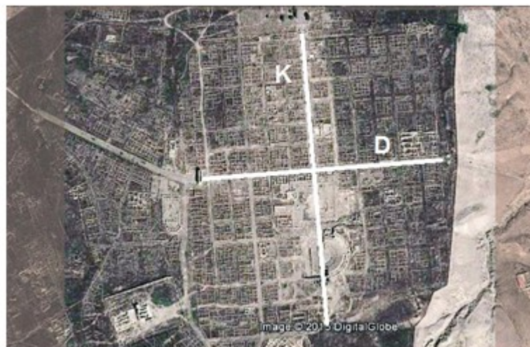
Figure 2 – Another Roman colonial town as seen in a Google Earth image. It is Timgad, in the Aurès Mountains of Algeria, founded by Emperor Trajan around AD 100, with the name Colonia Marciana Ulpia Traiana Thamugadi. Located about 35 km East of the town of Batna, the ruins are clearly showing the grid plan, based on Decumanus (D) and Kardo (K). Here, the Decumanus is at a small angle with the East-West cardinal direction [4]. The arc of Trajan is at the west end of Decumanus.
