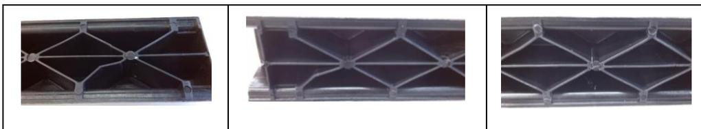
**Figure 5-44 different damage modes under torsion**
