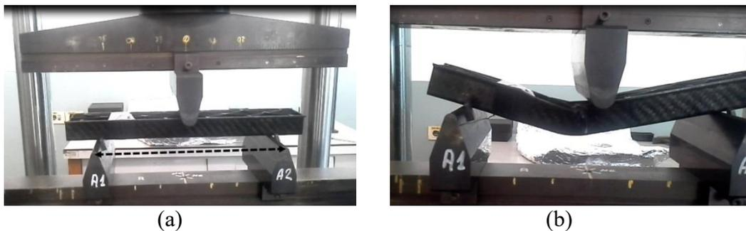
**Figure 5-2 Bending test configuration; (a) test starting point (b) ending point [6]**
