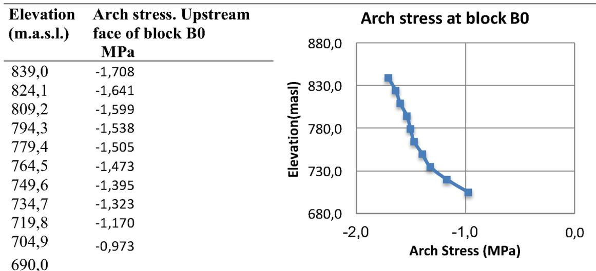
Figure 5: Arch stress. Upstream face at block B0
