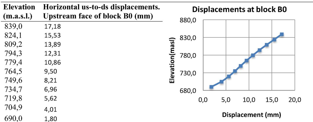
Figure 3: Horizontal us-to-ds displacement at block B0
