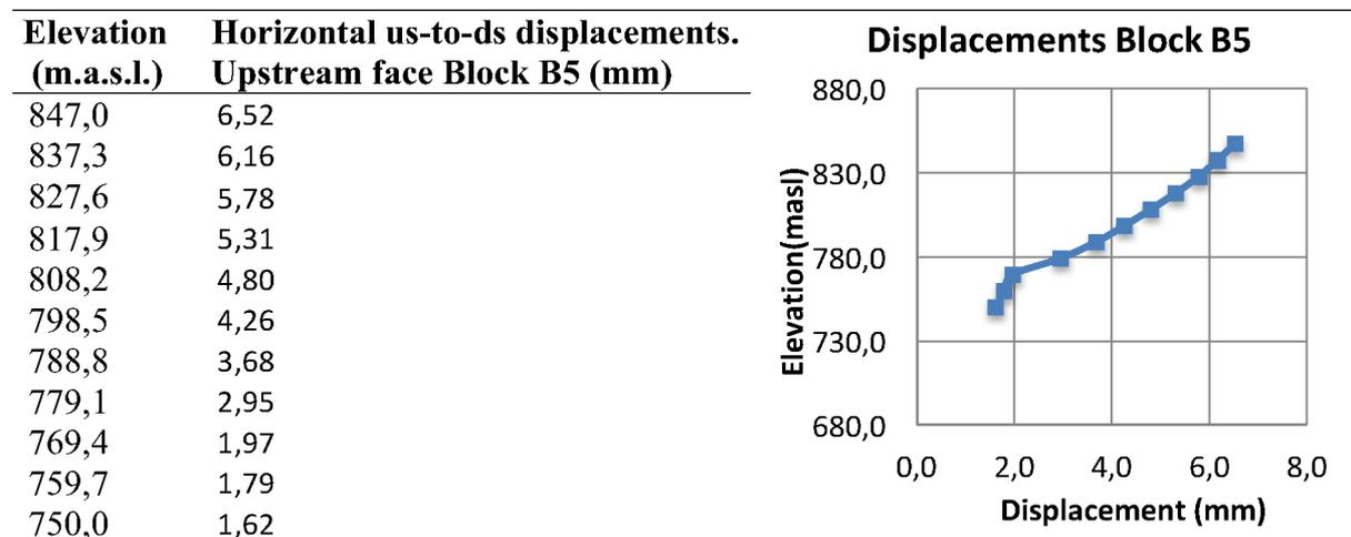
Figure 4: Horizontal us-to-ds displacement at block B5
