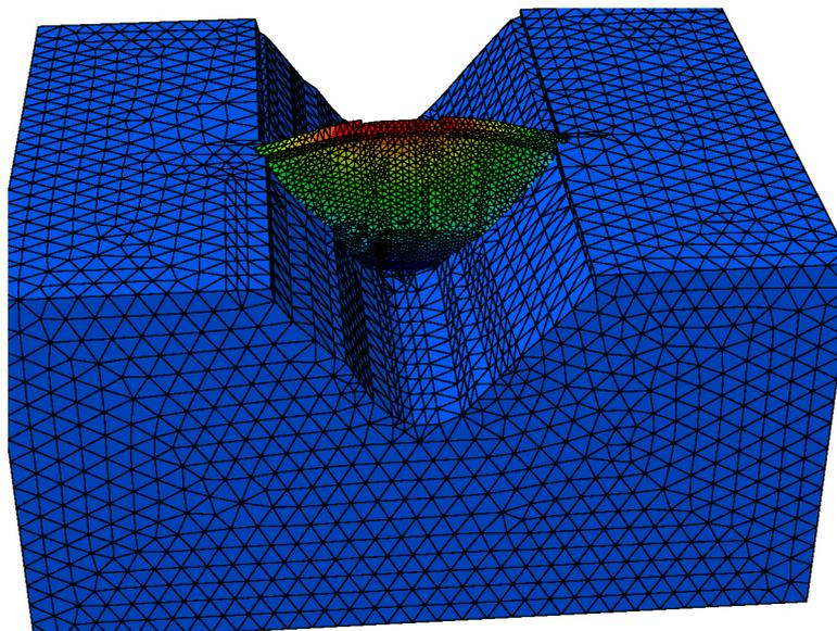
Figure 12: 1<sup>st</sup> eigenmode of linear model
