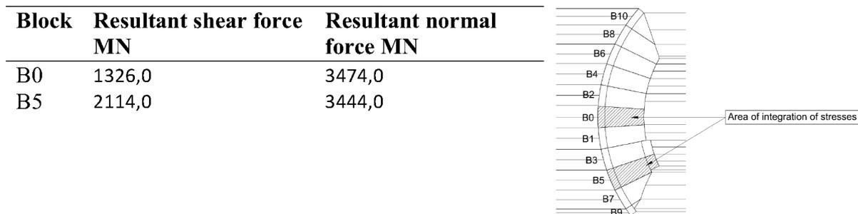
Figure 6: The resultant shear and normal forces
