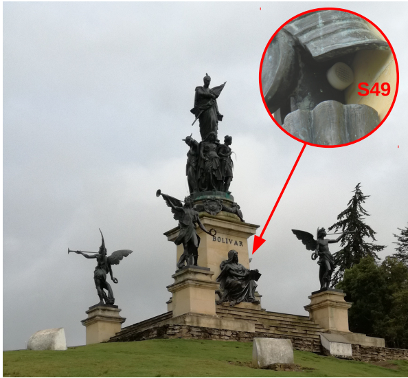
Fig. 4. Placement of the sensor node S49 on the Von Miller Monument (Punto de Boyacá).
