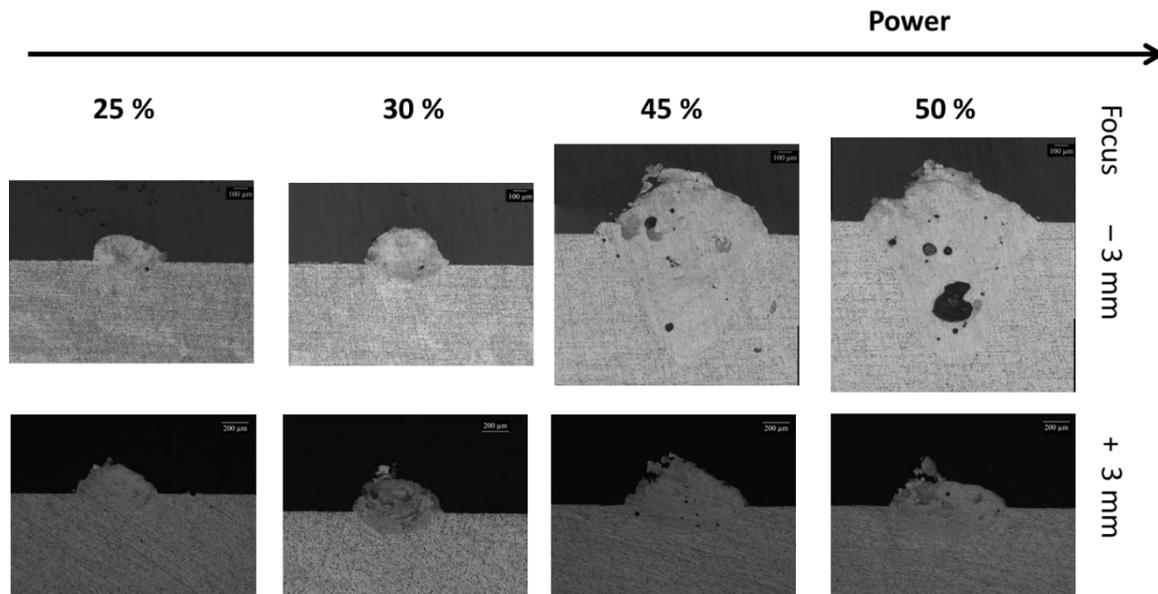
Fig. 6 Cross-section micrographs of some DED SSTs.
