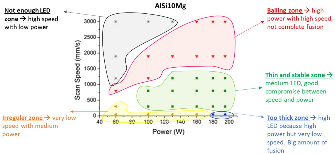
Fig. 4 LPBF process window for AlSi10Mg SSTs.
