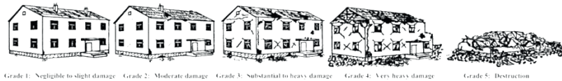
Figure 1. Classification of damage to masonry buildings from EMS-98 scale (European Macroseismic Scale) (Grunthal, 1998).
