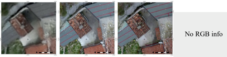
Figure 16a. Comparison, on a small area, between used platforms and sensors: eBee, average GSD of 5 cm/pixel (left); DJI Phantom, average GSD of 2.18 cm/pixel (center left); fusion model, average GSD of 0.92 cm/pixel (center right); no RGB data from Zeb1.
