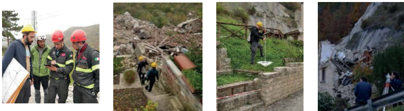
Figure 4. Survey operation during the setting up of the topographic measurements. A moment of the aerial markers planning and placing on ground with fire fighters (left). Global Navigation Satellite System (GNSS) measurements on target disseminated in more or less accessible areas in the neighborhood of the damaged building, with the Leica System 1200 GNSS receiver (center left and right), Leica TS06 total station topographic survey (right).
