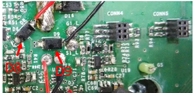
Fig. 6. Detail of the PCB board with the two diodes very close to each other.
