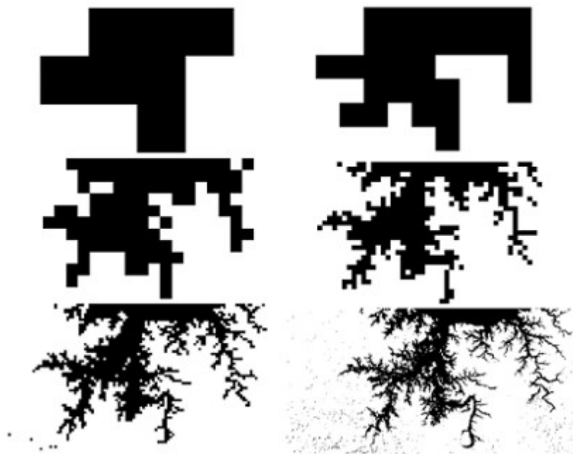
Figure 2: Using the Pixelize filter of GIMP we have a series of binary images that we use for evaluating the fractal dimension of the coastline.
