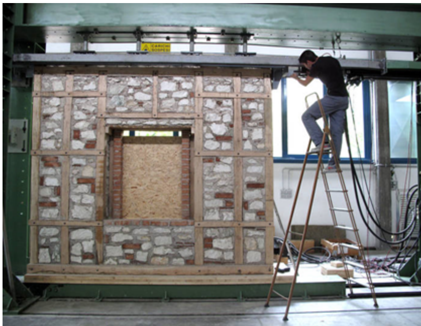
Figura 3 - Ricostruzione di parete antisismica in muratura baraccata, presso i laboratori del CNR-IVALSA - Reconstruction of an "ancient" seismic safety masonry building technology at the CNR-IVALSA laboratories.
