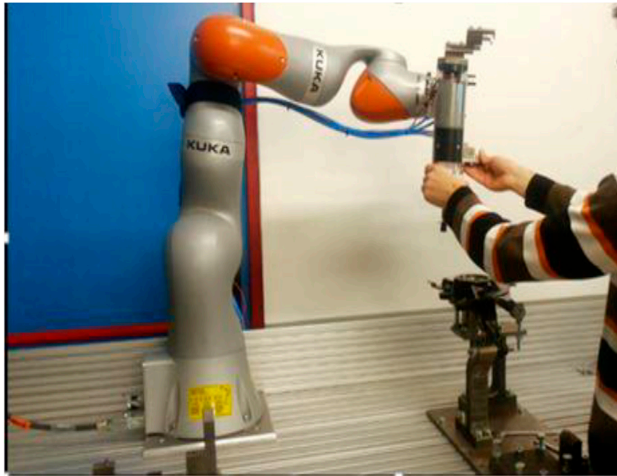
Figure 16. Human-robot collaboration with the hand-guided (HG) method during the assembly process of a brake disc.
