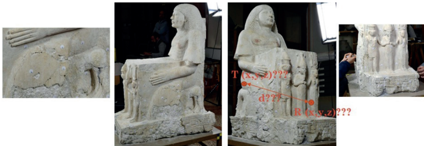
Figure 1. (Left) Worrying state of deterioration of the statue with visible fractures, (right) the ultrasonic measurements to reconstruct the fracturing state of the statue needs to know several vector size between points on the damaged surface.
