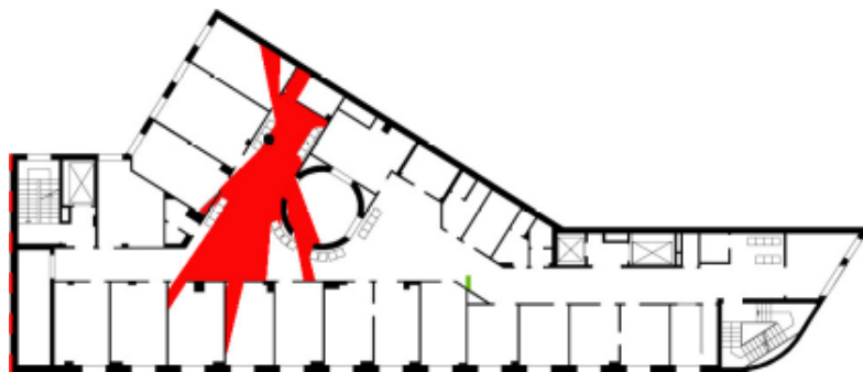
Figure 4 - Application of the "Visibility from the previous step of the path" indicator, used to verify the route clarity (Table 2). The use of the isovist shows how the acceptance waiting area is only partially visible from the previous step of the path (reception).
