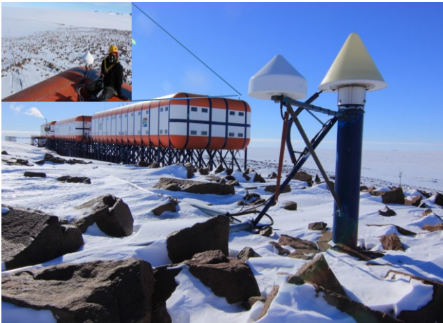
Figure 1. Antennas of the co-located GNSS receivers at SANAE, the South African Polar Research base in Antarctica. In the foreground is the antennas of the GPS and Novatel Scintillation receivers, and on the roof of the base (insert) is the antenna shared by the Septentrio PolaRxS PRO GNSS receiver and the software-based GNSS data acquisition system, comprising the 4tuNe front-end and a Software Defined Radio (SDR) GNSS receiver.
