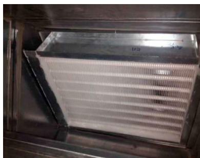
Figure 1.Coated Finned coil for heat and mass transfer Figure 2 Zoom of the SAPO 34 coating mass transfer
