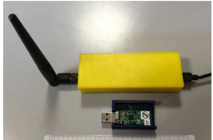
Fig. 5. Picture of two prototypes of receivers designed to be powered by the USB port of a PC.
