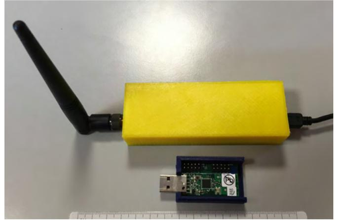
Fig. 5. Picture of two prototypes of receivers designed to be powered by the USB port of a PC.
