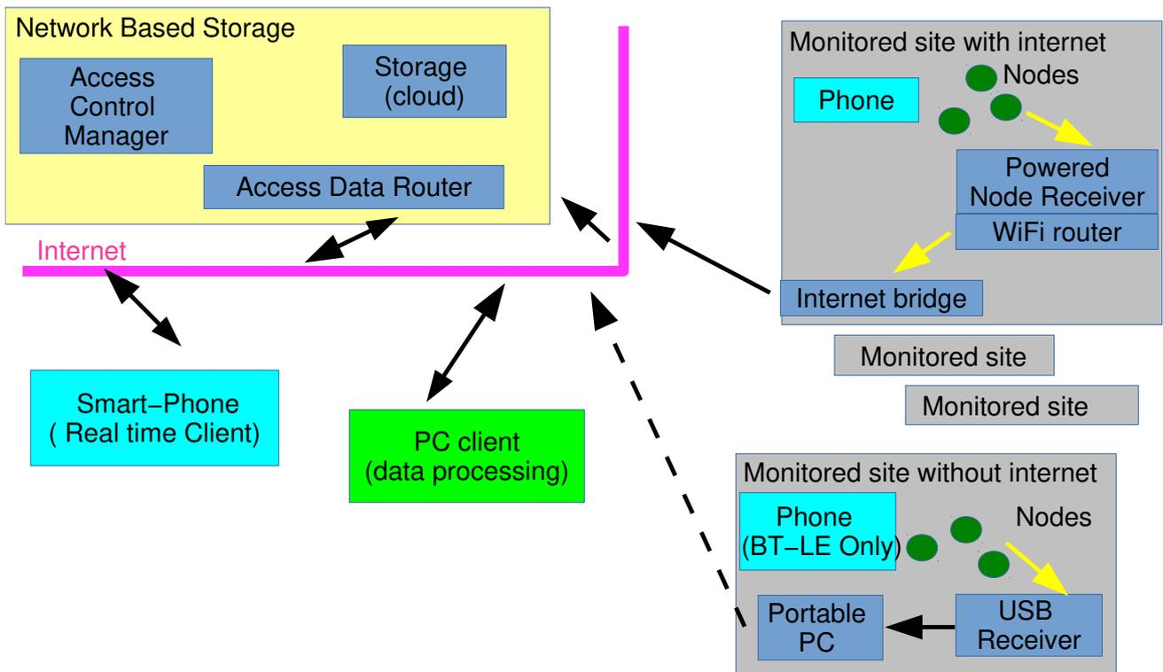
Fig. 1. Block diagram of the proposed measuring architecture.
