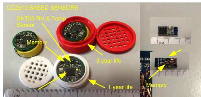
Fig. 3. Measuring node prototypes arranged with different technologies.
