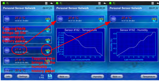
Fig. 6. Pictures of the virtual panel arranged on a smart-phone by using the \mu Panel technology and which is generated by the on-line receiver
