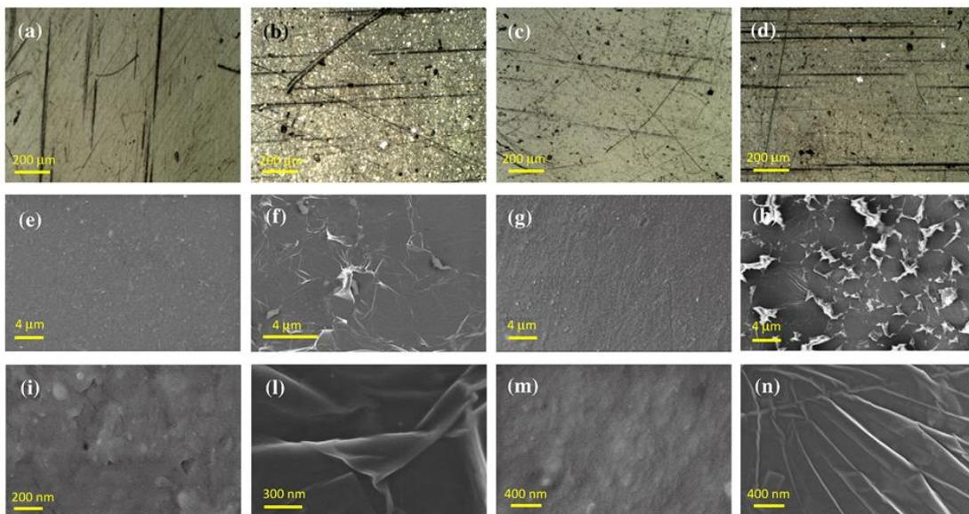
Figure 1. Surface images of the samples. Optical microscope of uncoated ABS (a), coated ABS (b), uncoated PC-ABS (c) and coated PC-ABS (d). SEM images of uncoated ABS (e), coated ABS (f),
