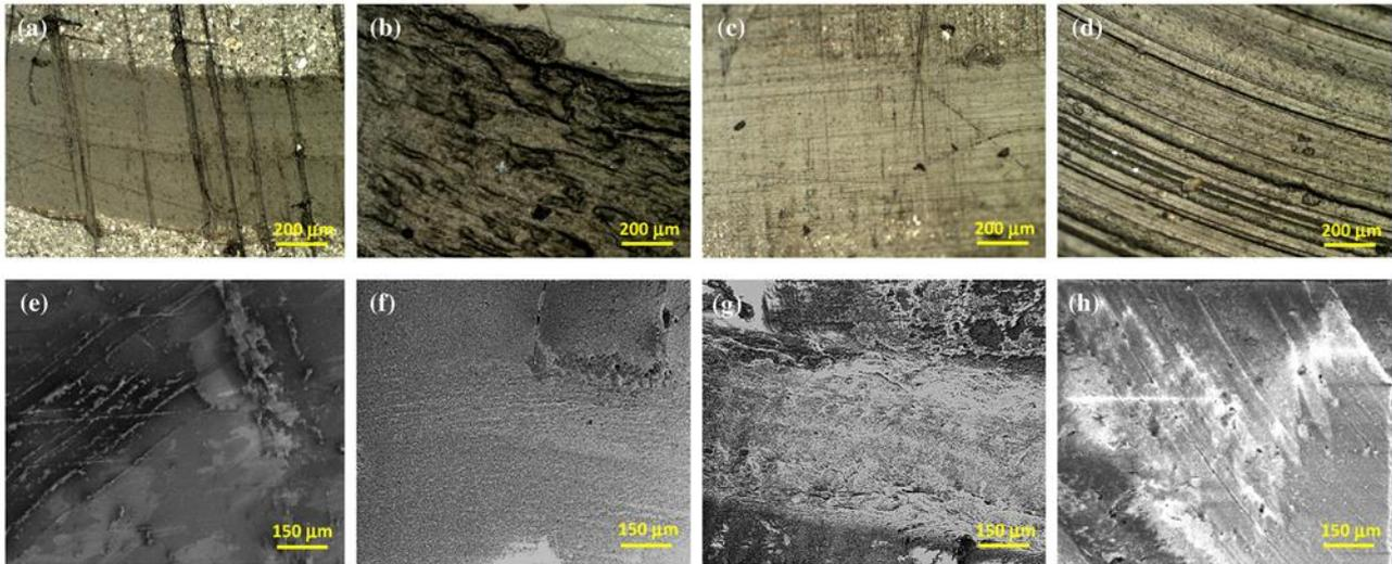
**Figure 9: Surface images of the tracks of the coated materials at different sliding distances. Optical microscope of the coated ABS sample after 0.5 m (a), coated ABS after 200 m (b), coated PC-ABS after 0.5 m (c) and coated PC-ABS after 200 m (d). SEM images of coated ABS after 0.5 m (e), coated ABS after 200 m (f), coated PC-ABS after 0.5 m (g) and coated PC-ABS after 200 m (h).**
