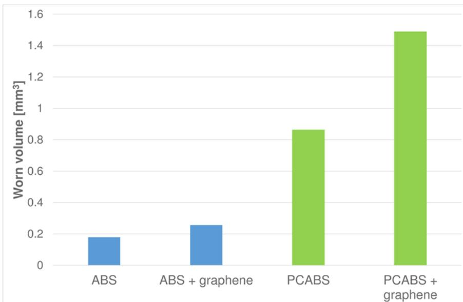
Figure 2. average worn volume in coated and uncoated samples after 200m sliding distance.
