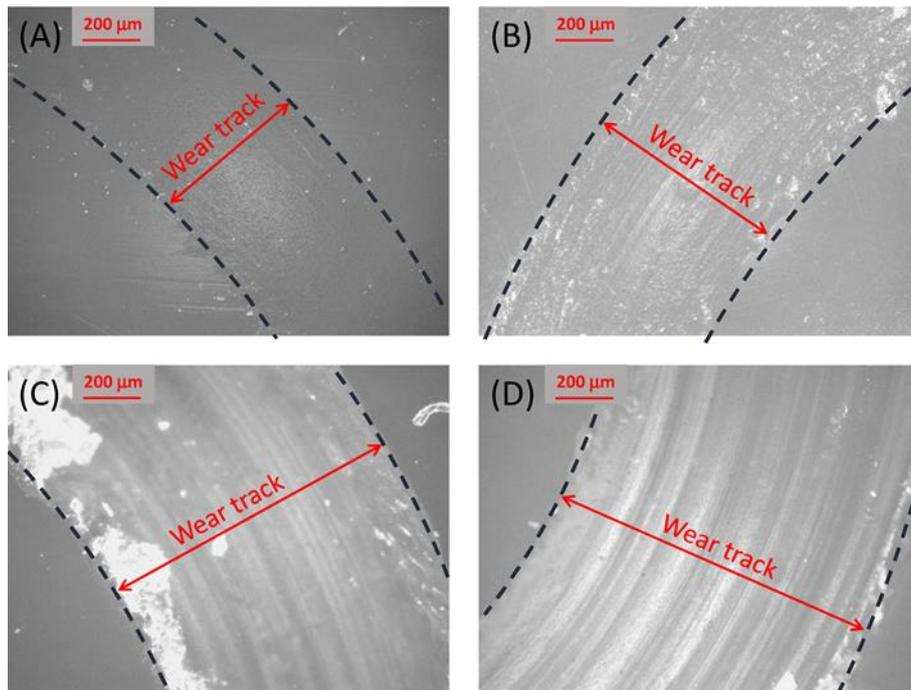
**Figure 3. Optical microscope images of samples after test 1(200m travelled distance): (A) uncoated ABS; (B) coated ABS; (C) uncoated PC-ABS; (D) coated PC-ABS. The scale bars are all 200µm**
