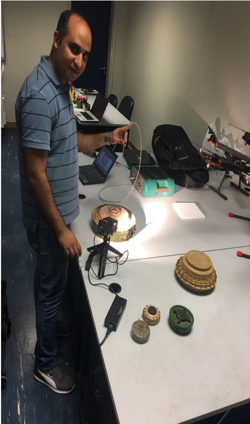
Figure 31: Acquisition of the reflectance spectrum of TM-46 landmine
