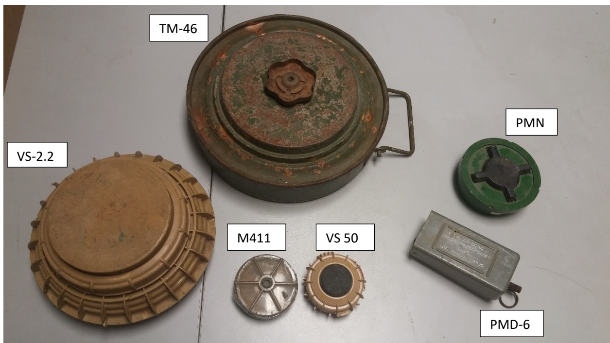
Figure 30: Samples of landmines used for acquiring their reflectance spectra
