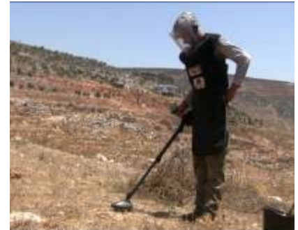
Figure 4: Landmine detection with metal detector
