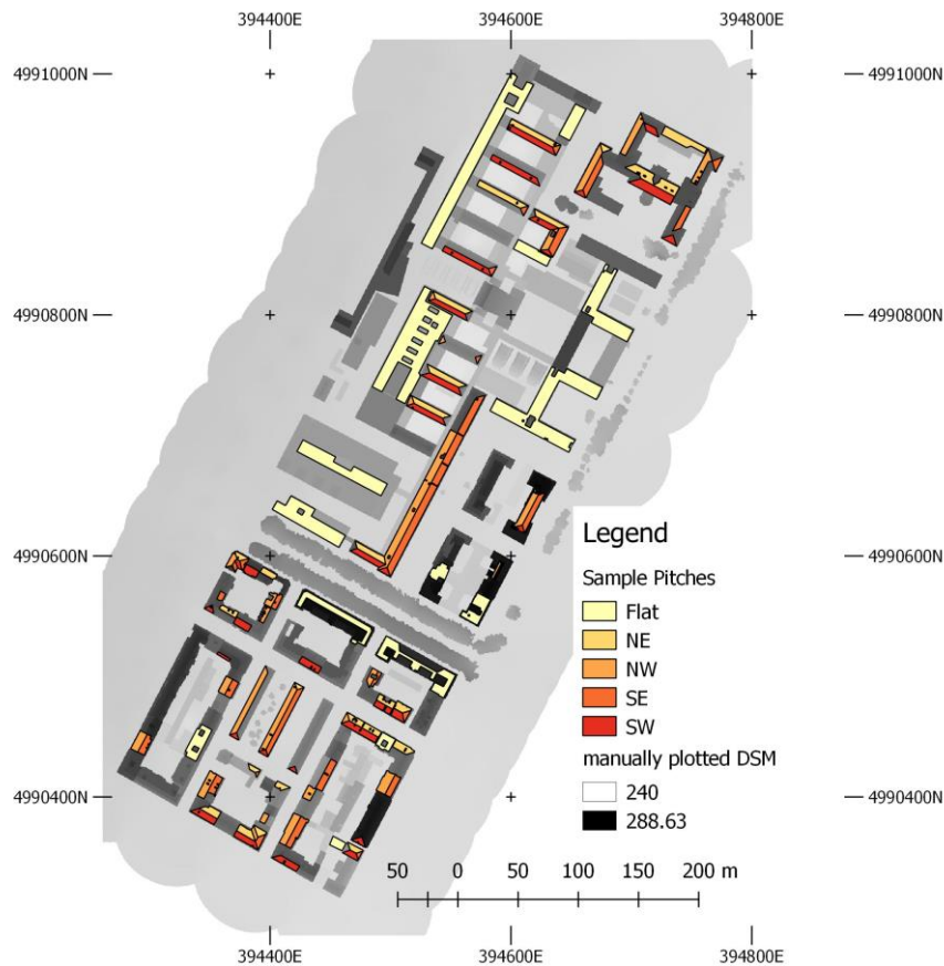
Figure 13 – Map of the roof pitches sample considered for extracting the raster values and performing the analyses.
