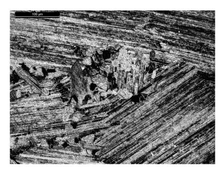
Figure 202c: near lamellar microstructure after heat treatment at 1360°C for 2 h.
