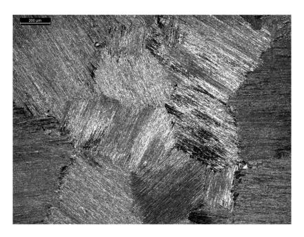
Figure 203a: near fully lamellar microstructure after heat treatment at 1365°C for 2h.
