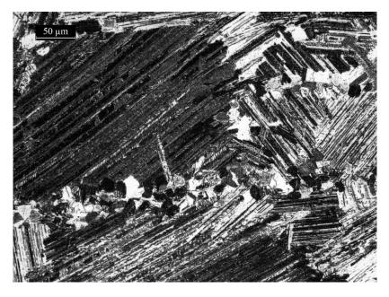
Figure 212 c: near lamellar microstructure after heat treatment at 1360°C for 1 h.
