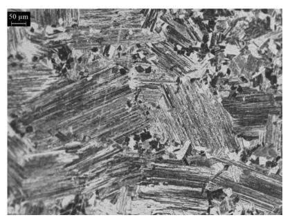
Figure 222: Duplex microstructure of the wheel thinner blade after the heat treatment at 1355°C for 1 h.
