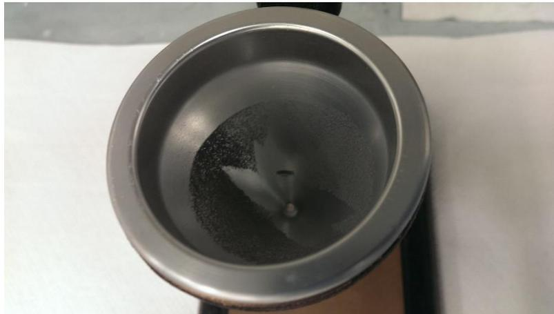
Figure 90: Powder stuck on the flowmeter walls
