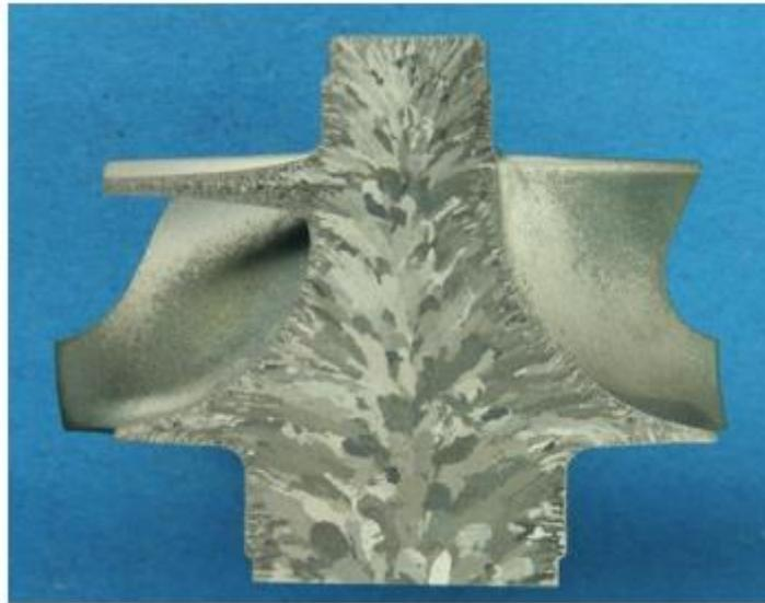
Figure 207: Macrostructure of the wheel produced by DAIDO steels.
