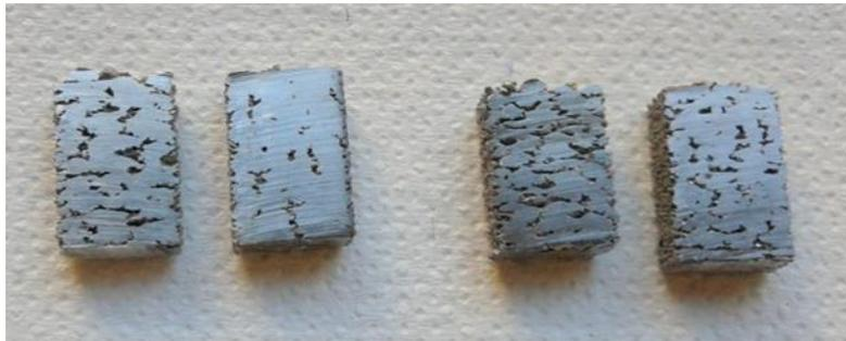
Figure 105: specimens from 13 to 16 with a high defects amount
