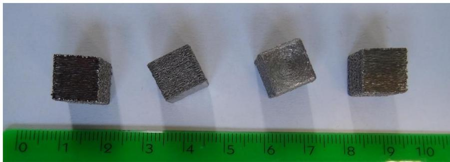
Figure 193: preliminary RNT650 test specimens produced by EBM
