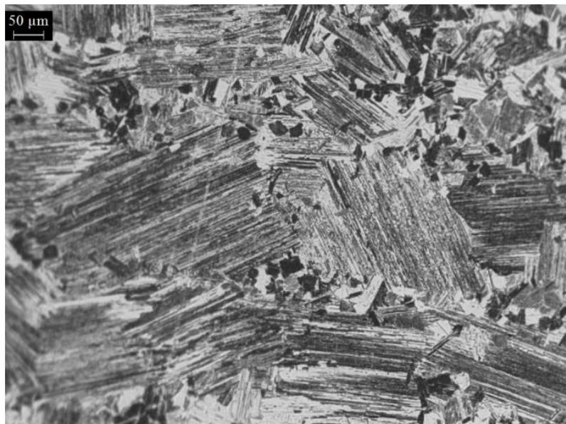
Figure 222: Duplex microstructure of the wheel thinner blade after the heat treatment at 1355°C for 1 h.
