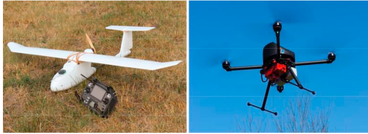
Fig. 1 An example of fixed and rotary wing model (MAVTECH Agri 1900 and Q4L (Micro Aerial Vehicles Technology, 2017)).
