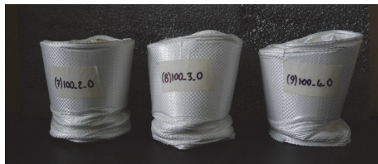
Fig. 7. Side view of the PURE tubes with the diameter of 100 mm at the end of the crush test. From left to right the wall thickness increases.
