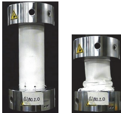
Fig. 3. Hybrid specimen under quasi-static compression before (on the left) and after (on the right) the test.
