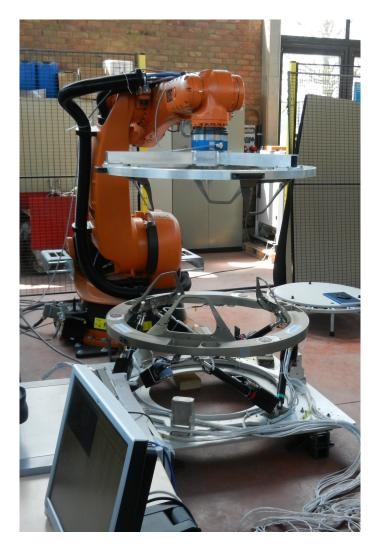
Fig. 2.29 Testing of the IBDM in Leuven, Belgium in 2012 (credit: ESA)
