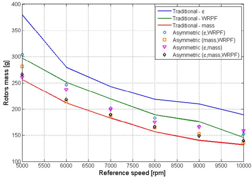
Figure 63: Multi objective optimization results: rotors mass
