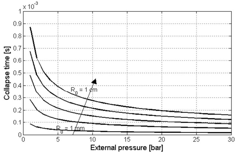
Figure 5: Example of cavitation bubbles collapse time
