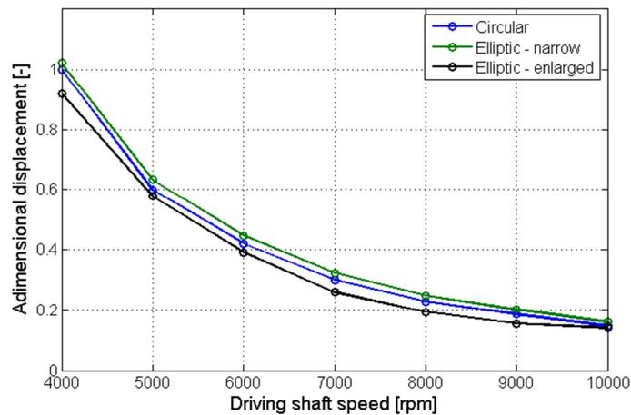
Figure 51: Maximum displacement for circular and elliptic profiles
