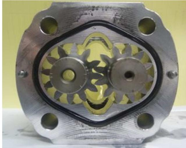
Figure 7: An external spur gears pump<sup>2</sup>
