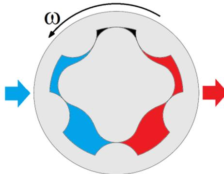
Figure 1: Simple scheme of a gerotor pump
