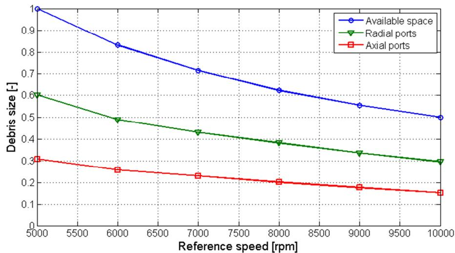
Figure 46: Maximum size of the expelled particles
