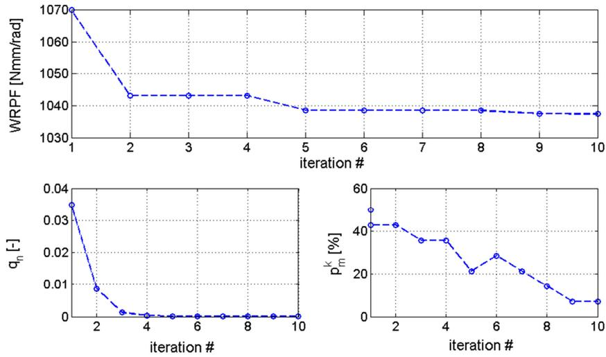
Figure 56: Algorithm behavior for  $n = 5000$  rpm, WRPF optimization
