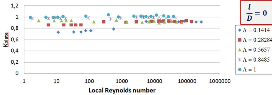
Figure 84: Variation of  $K_{plate}$  with  $\Lambda$ ,  $\alpha = 45^\circ$
