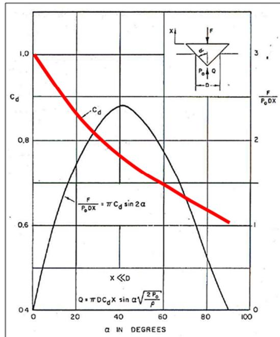
Figure 75: Discharge coefficients according to Von Mises' theory
