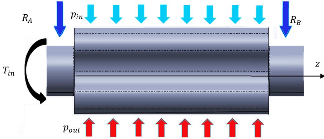
Figure 37: Static equilibrium of the inner rotor shaft
