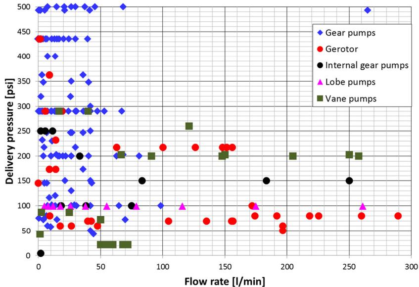
Figure 12: Catalogues data – delivery pressure vs flow rate
