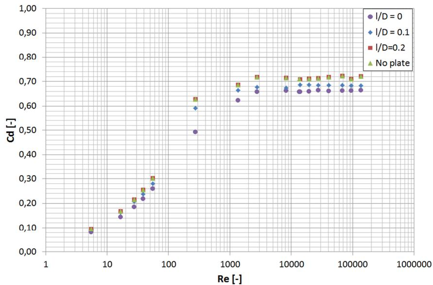
Figure 83: Variation of  $C_d$  with  $l/D$ ,  $\alpha = 45^\circ$
