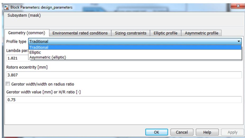
Figure 39: Input mask for the pump design routine
