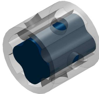
Figure 22: Concept of radial ports for gerotor pumps
