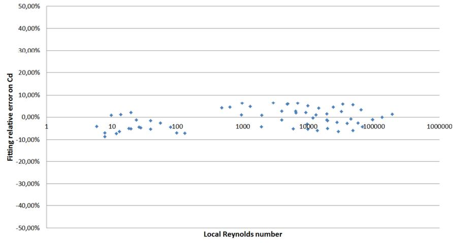
Figure 80: Relative error on  $C_d$ ,  $\alpha = 30^\circ$
