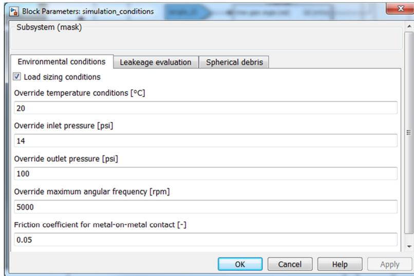
Figure 40: Input mask for the pump simulation routine
