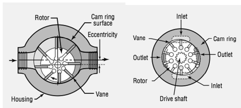
Figure 10: Unbalanced and balanced vane pumps<sup>5</sup>
