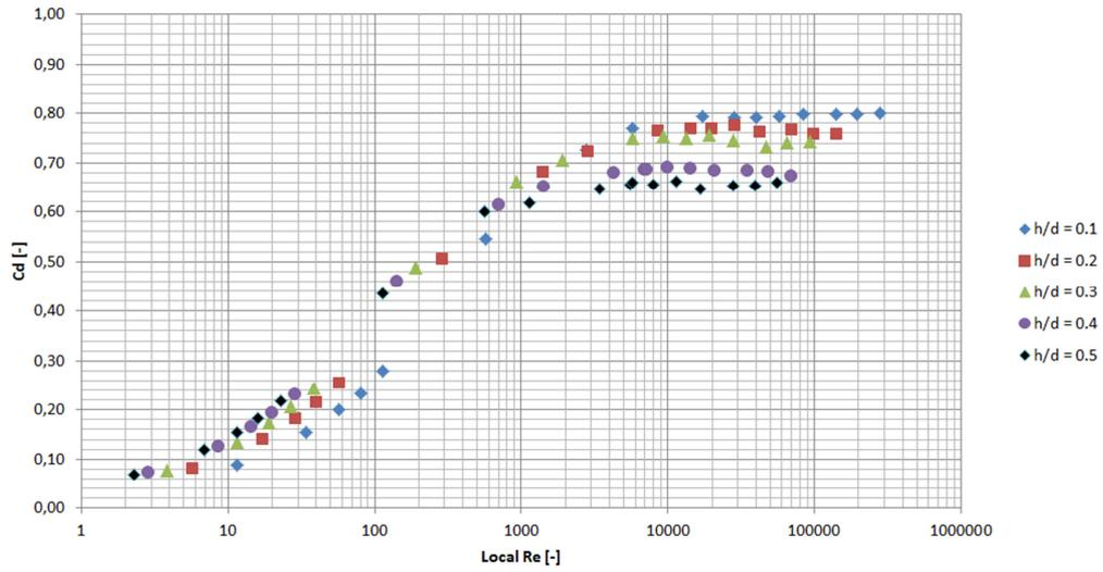
Figure 76: CFD results: discharge coefficient,  $\alpha = 20^\circ$
