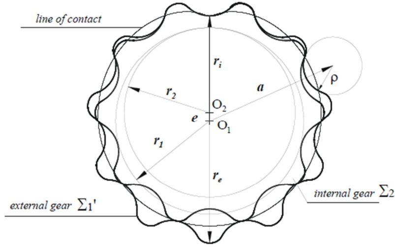
Figure 14: Geometrical parameters for epitrochoidal gerotor pumps
