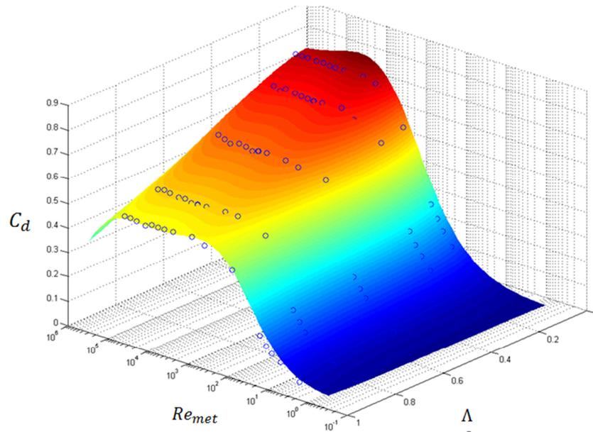
Figure 79: Polynomial fitting vs CFD results,  $\alpha = 45^\circ$
