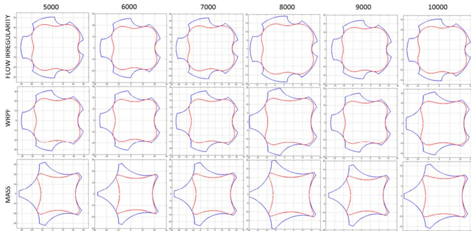
Figure 59: Optimized cycloidal profiles in the 5000 – 10000 rpm range
