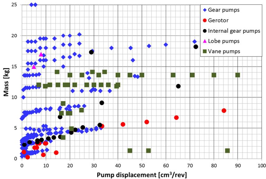
Figure 13: Catalogues data – pump’s mass vs displacement
