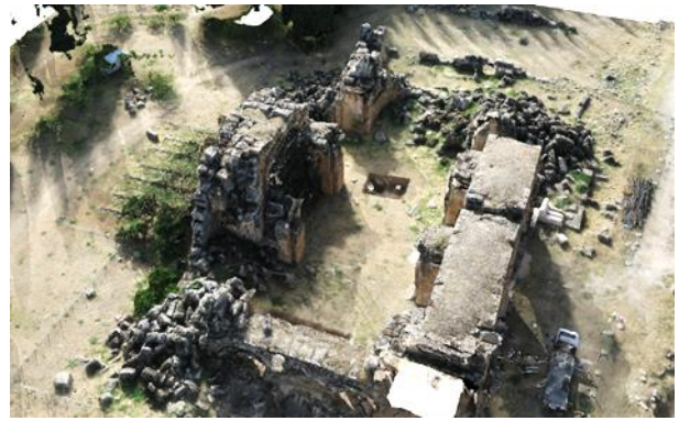
Figure 17: A 3D view of the textured DSM processed from the Terme-Chiesa flight.
