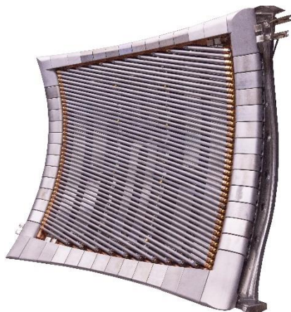
Fig. 3. Real antenna model installed on AUG
