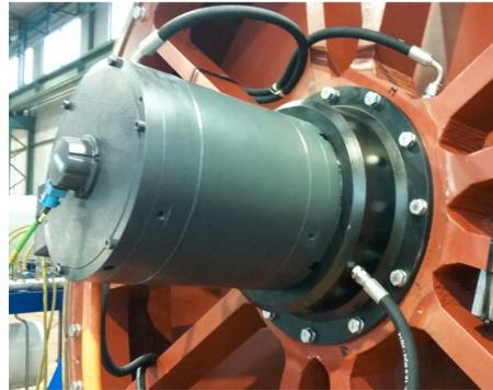
Figure 4.13 The gyroscope: flywheel motor.
