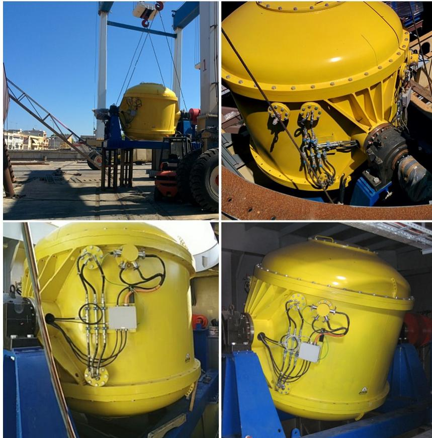
Figure 4.5 The floater: first gyroscope group installation.
