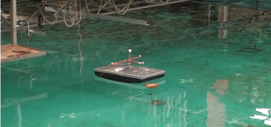
Figure 2.17 Hydrodynamics Tank Tests. Floater moored to the tank floor. 6 DOF analysis.
