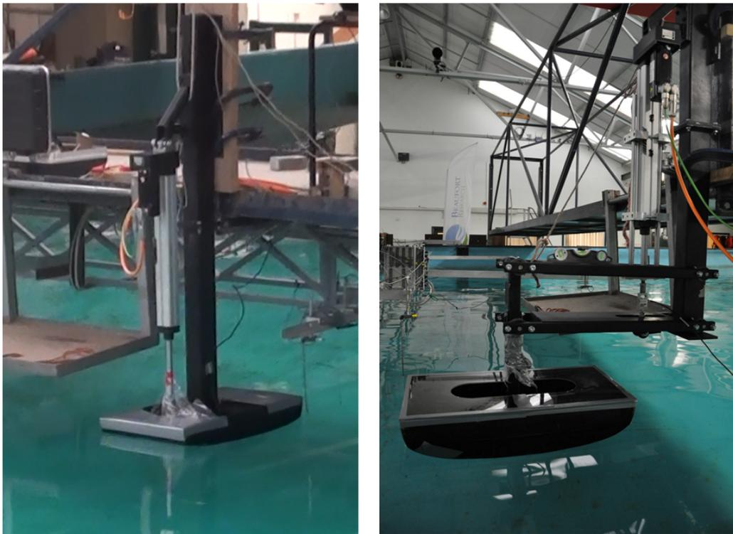
Figure 2.14 Hydrodynamics Tank Tests. Pitch and Heave test rig installed in HMRC tank in Cork (Ireland), 2014.
