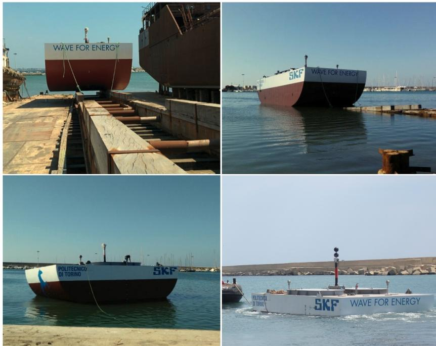
Figure 4.6 The floater: launch and ballast filling operations.
