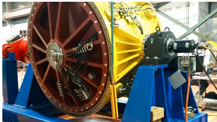
Figure 4.16 The gyroscope: flywheel lubricating system, oil recovery pump and rotary hydraulic joint.
